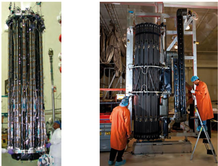
Figure 5.12. LDR in stowed configuration. Left: Harris Corp.; Right: Northrop Grumman.
