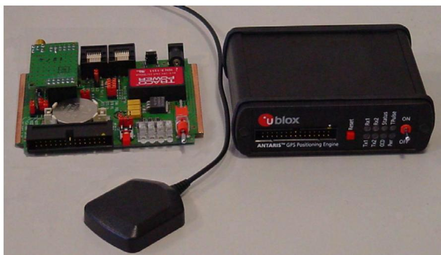
**Figure 3.8:** The uBlox Antaris GPS receiver. The picture show the power supply and interface PCB (left) with the GPS module plugged on the left side of the board. The enclosure of the electronics is shown on the right. The patch antenna is shown in the foreground.
