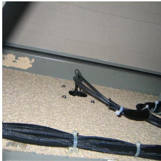
b) Cables leading into the socket (view from inside the tram).
