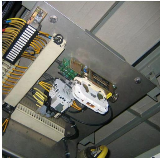
d) Contactor and fuse as a safety measure in the tram.
