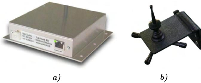
*Figure 3.12:* The GSM communication system consists of a GPRS/GSM gateway (*a*) and an antenna (*b*).
