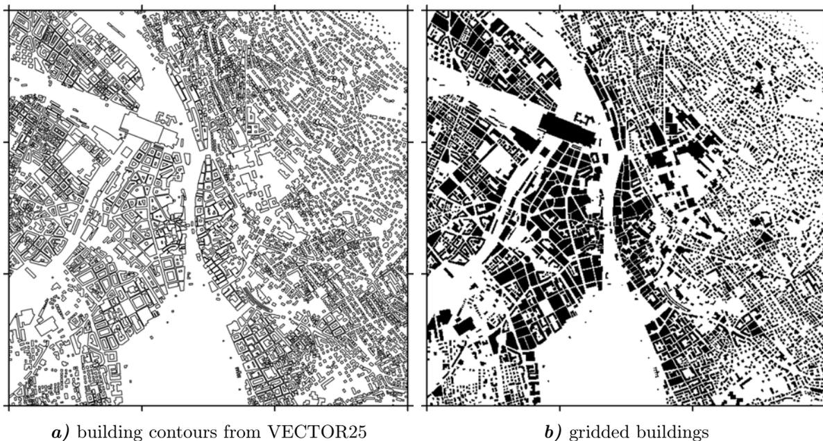
**Figure 6.3:** The building geometry in the 3.3 km<sup>2</sup> study area (**a**) were extracted from the VECTOR25 data set. The vector data was gridded with 5 m mesh width (**b**) and included in the dispersion calculations.
