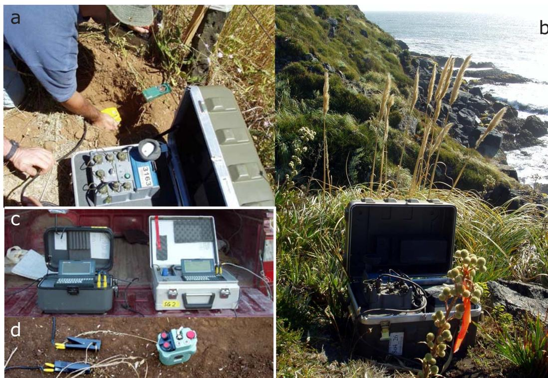
**Figure 2.4.:** Receiver stations and shooting equipment. Panel a shows the buried and oriented 3-component geophone and the EDL recording unit in a weatherproof box. The picturesque last receiver station 955 at the Pacific Ocean is shown in b. Panel c shows two similar boxes to record the exact shot times, e.g., with pliers around the ignition lead, not yet connected to the trigger box (d). Image courtesy of C. Krawczyk.
