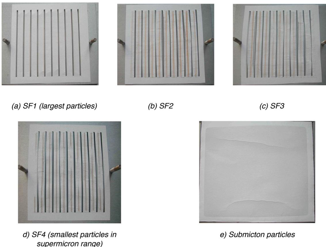
Fig. 3.3: Example of slotted (SF1–4) and backup (3(e)) filters after 24 hours of sampling of aerosol containing dust from the Sahara
