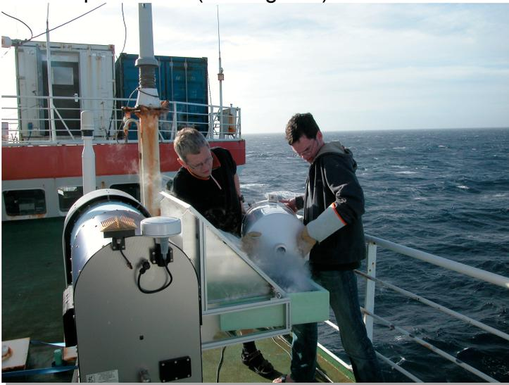
*Fig. 4.1: Filling of liquid nitrogen for calibration of the HATPRO microwave radiometer after departure from Cape Town*
