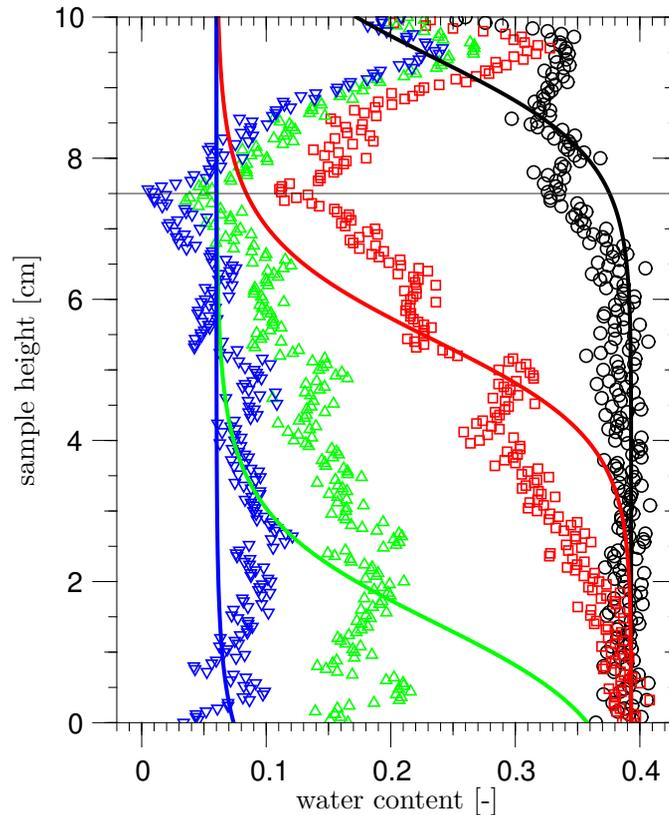
**Fig. 3.** Measured (symbols) and simulated (solid lines) vertical water content profiles assuming a homogenous sample. The matric head at the lower boundary was 8 cm (black), 12 cm (red), 16 cm (green) and 20 cm (blue) for the shown profiles. The hydraulic parameters were estimated by inverse modeling of the MSO experiment. Above the horizontal line ( $z=7.5$  cm) the measurements are affected by changes in the sample surface that leads to unreal water content values.
