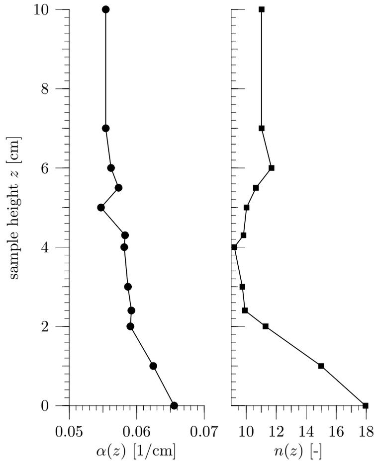
**Fig. 4.** Fitted van Genuchten parameters  $\alpha(z)$  and  $n(z)$ .
