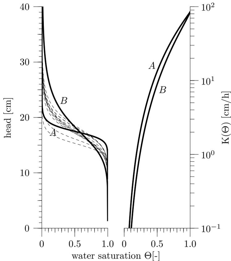
**Fig. 6.** Water retention curve (left) and hydraulic conductivity (right) for the two flow directions. Parameters for the respective curve A and B (solid lines) can be found in Table 1. The dashed water retention curves are calculated from the values  $\alpha(z)$  and  $n(z)$  shown in Fig. 4.
