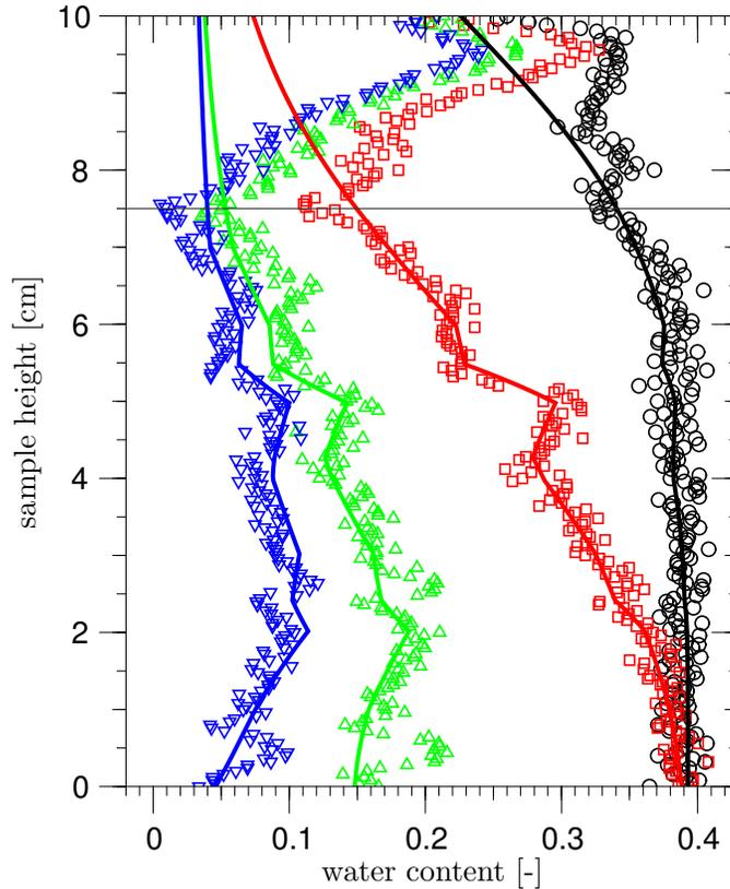
**Fig. 5.** Measured (symbols) and simulated (solid lines) vertical water content profiles assuming a heterogeneous sample. The matric head at the lower boundary was 8 cm (black), 12 cm (red), 16 cm (green) and 20 cm (blue) for the shown profiles. Above the horizontal line ( $z=7.5$  cm) the measurements are affected by changes in the sample surface that leads to unreal water content values.
