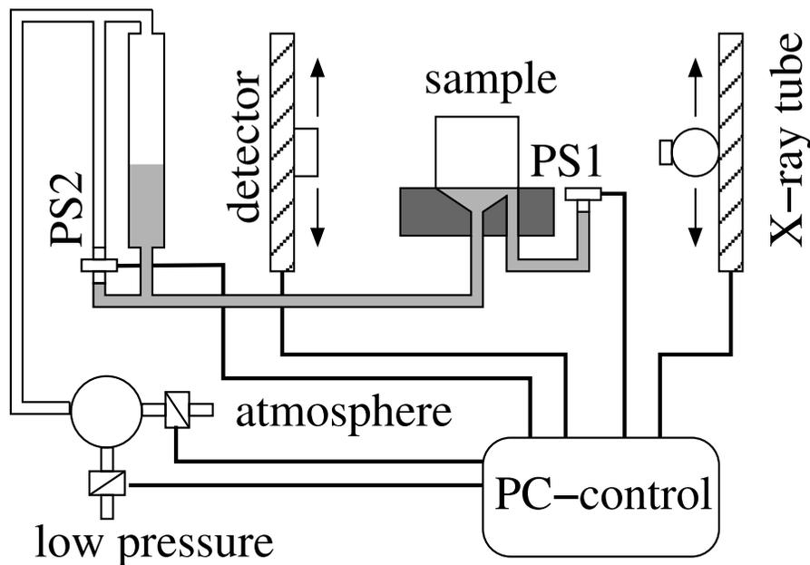
**Fig. 1.** Sketch of the experimental setup: The sample is placed between the X-ray source and the line detector, which both can be moved vertically. The pressure at the lower boundary is measured by the sensor PS1 and controlled by a computer. The water outflow is collected in a burette and measured using the pressure sensor PS2.
