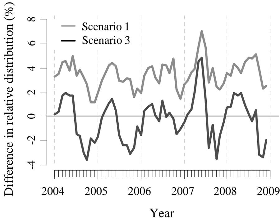
**Fig. 11.** Difference in relative contribution of the WWTPs to the total river flow between the model-based and empirical approaches (scenario 1 and scenario 3). The difference in contribution increases during flow recession periods.
