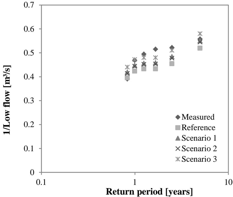
**Fig. 12.** Return period of hourly low flow extremes for the Grote Nete catchment between 2004 and 2008.
