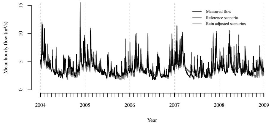
**Fig. 7.** Observed and simulated runoff series for model calibration and validation (= 0.25).
