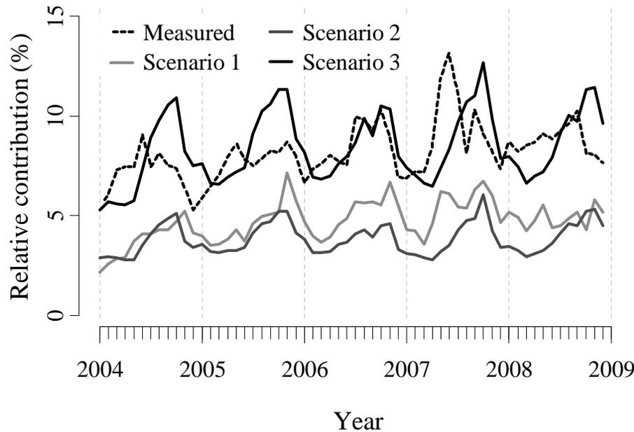
**Fig. 10.** Relative contribution (% monthly mean total flow) of the WWTPs to the total river flow. “Measured” refers to the empirical results obtained in Sect. 3.1.
