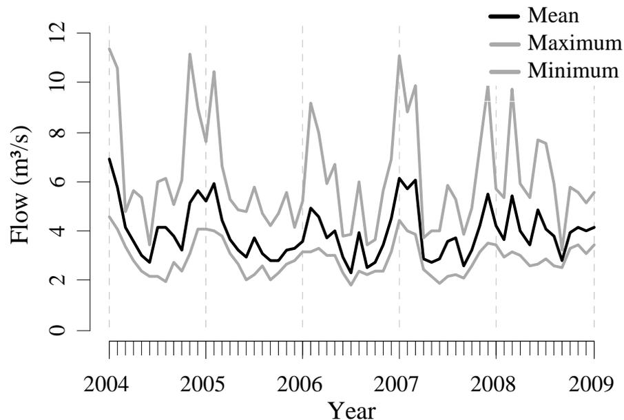
**Fig. 3.** Monthly mean, minimum and maximum of the daily measured flow (m<sup>3</sup> s<sup>-1</sup>) for the period 2004–2008 at the outlet (Varendonk) of the Grote Nete catchment.
