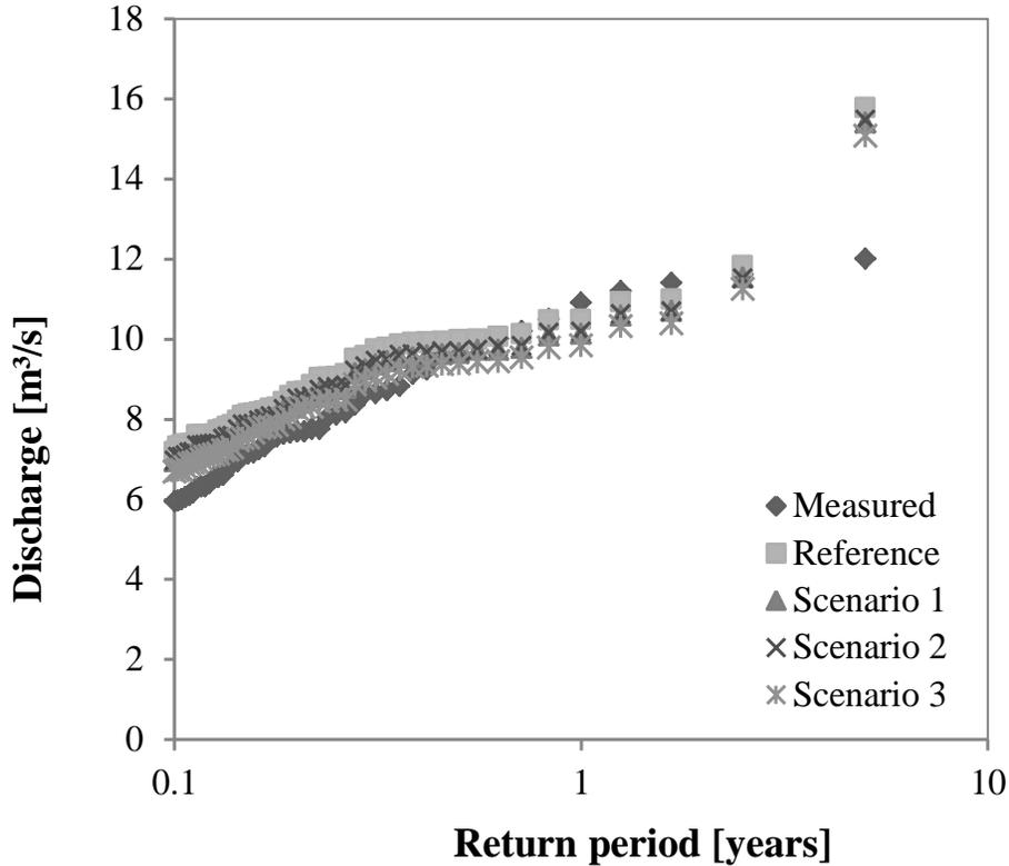
**Fig. 12.** Return period of hourly peak flow extremes for the Grote Nete catchment between 2004 and 2008.
