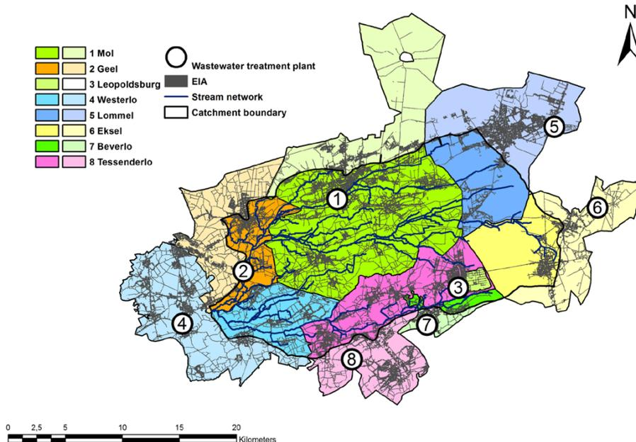
**Fig. 1.** Overview of the different WWTPs that are situated within the Grote Nete catchment (1–3) and the WWTPs that receive wastewater from impervious areas that are situated within the Grote Nete catchment but discharge in another catchment (4–8).
