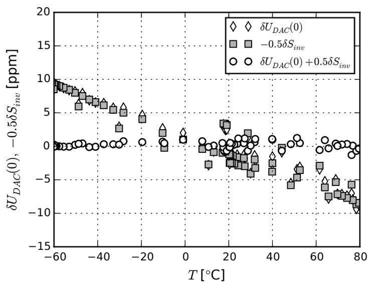
**Figure 6.** Temperature drift of the voltage reference inverter scale factor and the DAC zero offset.
