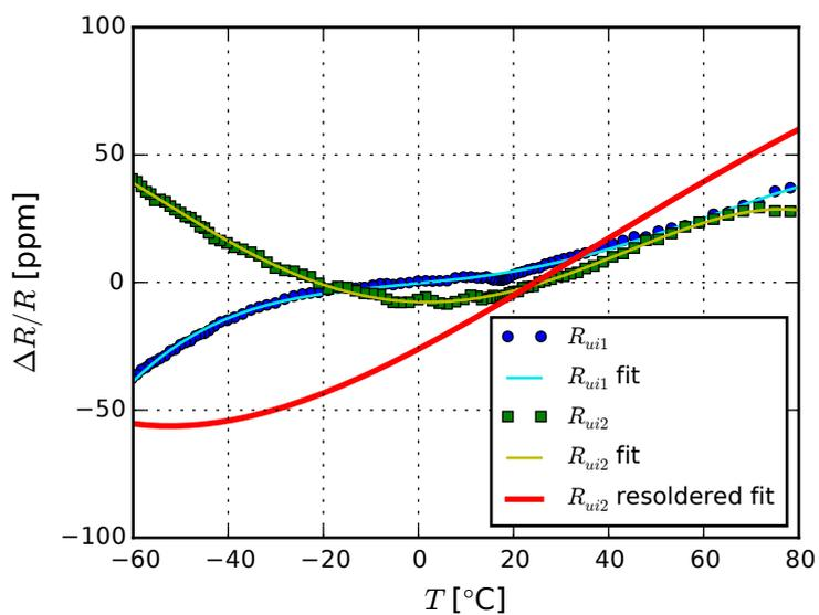
Figure 8. VSMP0805 resistors temperature dependences.
