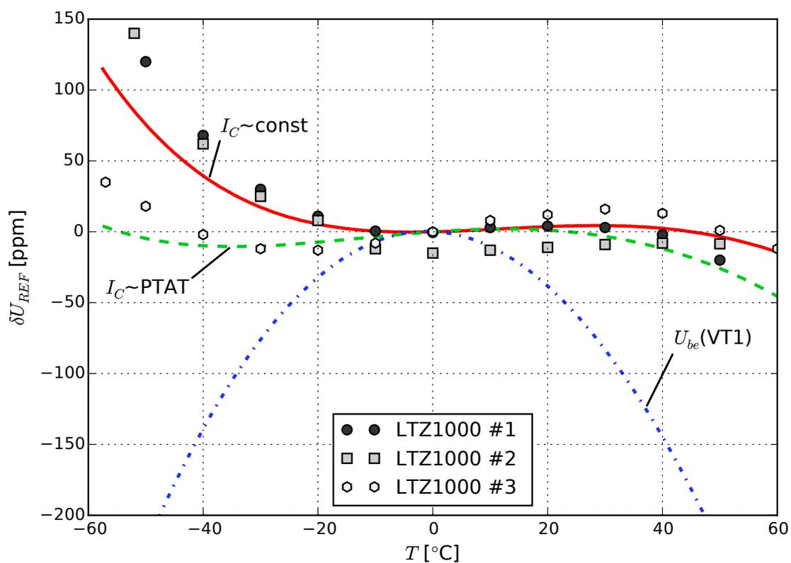
**Figure 2.** Temperature dependence of LTZ1000 reference voltage – simulated results (lines) and experimental data (marks).
