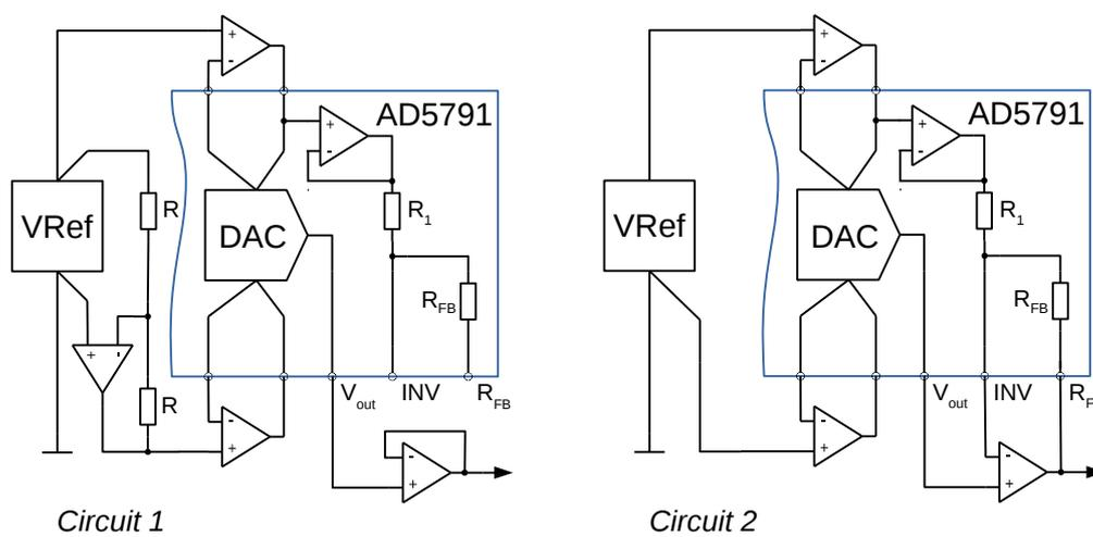
**Figure 5.** Digital to analog converter configurations.
