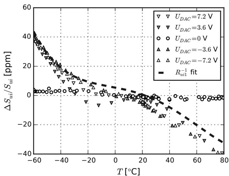
**Figure 7.** Temperature drift of the voltage-to-current converter transformation factor.
