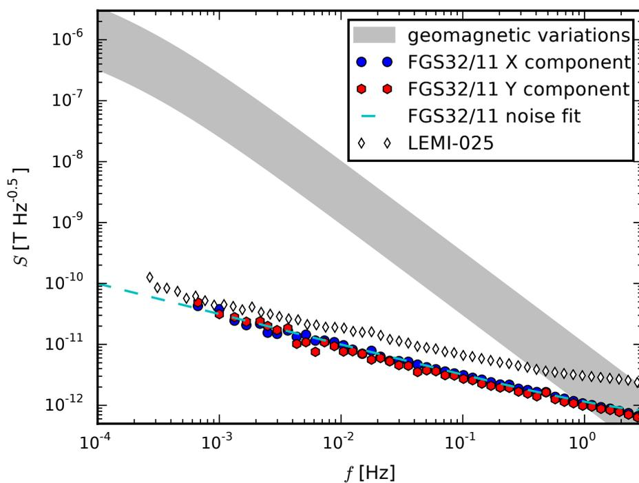
**Figure 1.** Noise spectra of flux-gate variometers.
