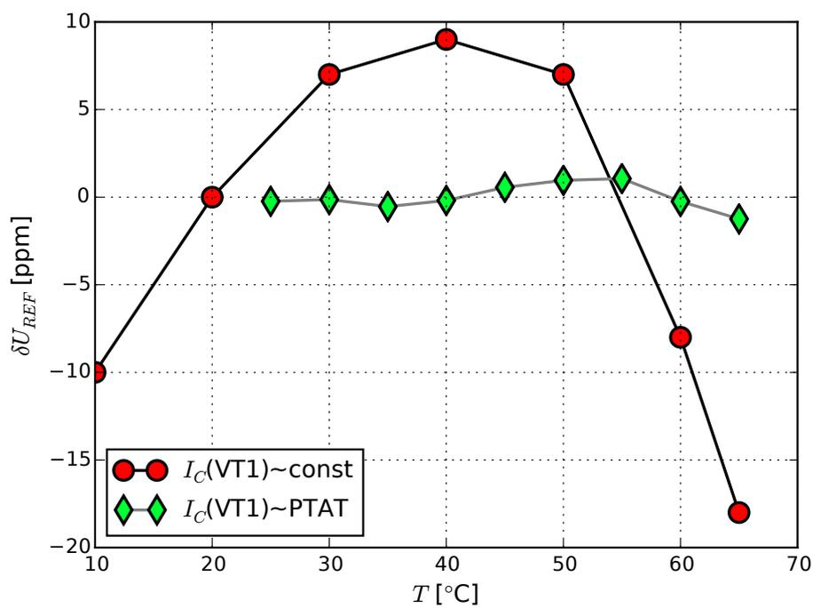
**Figure 4.** LTZ1000 voltage curvature correction.
