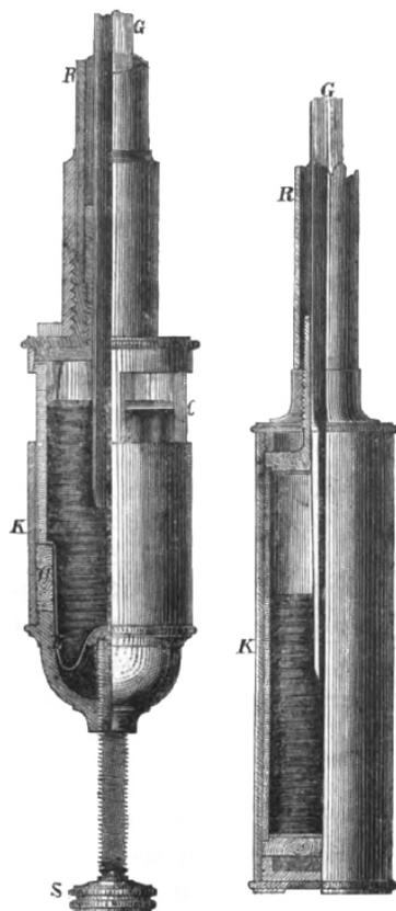
**Figure 2.** Drawing of the cisterns of a Fortin barometer (left) and of a fixed-cistern barometer (right). In the Fortin barometer a screw (indicated by the letter “S”) allows to adjust the level of the mercury in the cistern. From Jelinek (1869).
