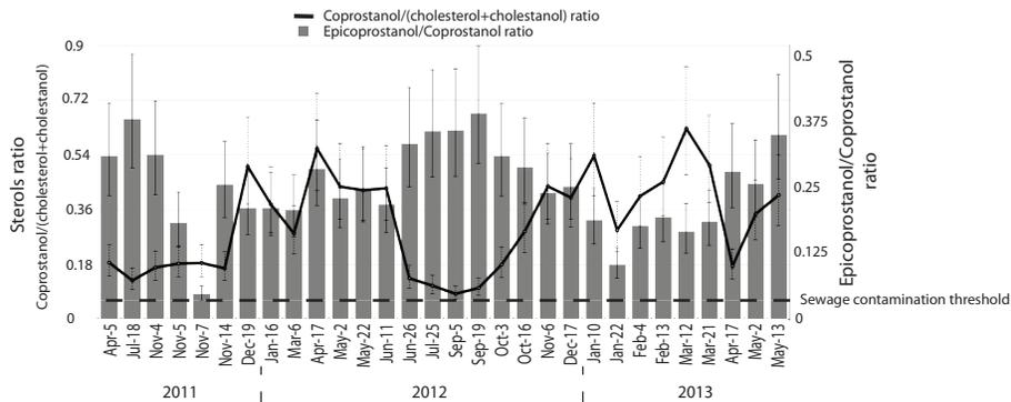
**Figure 6.** Coprostanol:(cholesterol + cholestanol) and epicoprostanol:coprostanol ratios of the different samples. Full error shown here incorporates the 14 % analytical standard error estimated for lipid quantification for all terms of the ratios. Contamination threshold is 0.06 (See Sect. 3.3.2).
