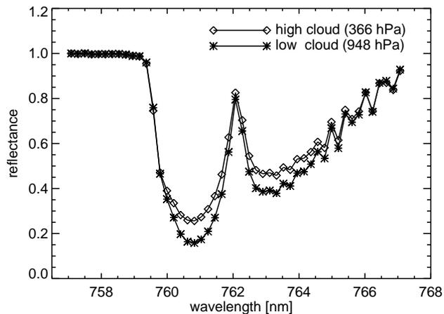
**Fig. 1.** Typical O<sub>2</sub> A-band spectra measured by GOME. The spectra are normalized at 758 nm to show the relative depth of the band for clouds at different heights.
