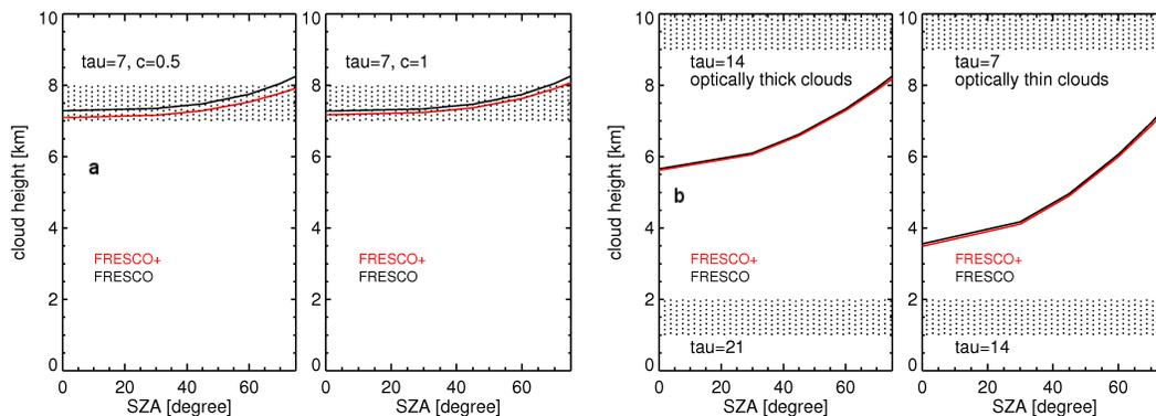
**Fig. 3.** FRESKO+ and FRESKO retrieved cloud heights using simulated spectra from a line-by-line multiple scattering model. Cases: **(a)** single-layer clouds, optical thickness  $\tau=7$ , cloud height at 7–8 km, and geometric cloud fraction  $c=0.5$  and 1. **(b)** two-layer clouds; cloud layer 1 at 9–10 km, cloud layer 2 at 1–2 km. Optically thick cloud:  $\tau_1=14$ ,  $\tau_2=21$ . Optically thin cloud:  $\tau_1=7$ ,  $\tau_2=14$ , geometric cloud fraction  $c=1$ .
