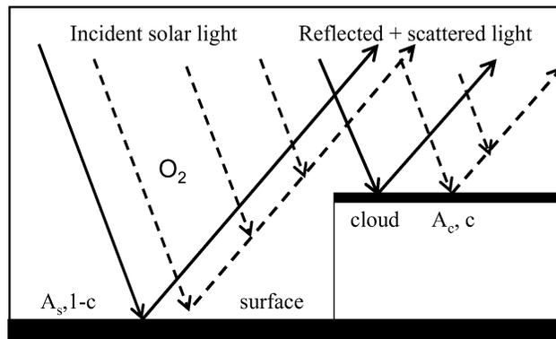
**Fig. 2.** Atmospheric radiation model used in FRESCO+. The cloud and surface are both assumed to be Lambertian reflectors. Three light paths are considered: (1) from sun to surface to satellite, (2) from sun to cloud to satellite, (3) from sun to atmosphere to satellite according to single Rayleigh scattering. (1)+(2): solid lines, (3): dashed lines. Along all three paths  $O_2$  absorption and Rayleigh scattering extinction are included in the forward model simulation.
