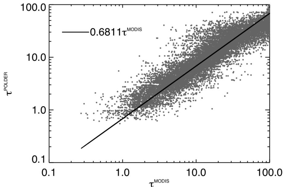
**Fig. 3.** Comparison of MODIS ( $\tau^{\text{MODIS}}$ ) and POLDER ( $\tau^{\text{POLDER}}$ ) ice cloud  $\tau$  retrievals for the granule in Fig. 2. The solid line corresponds to a fitting of  $\tau^{\text{POLDER}}$  with  $0.6811\tau^{\text{MODIS}}$ .
