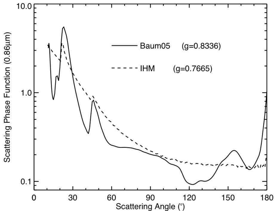
**Fig. 1.** The scattering phase functions and corresponding asymmetry factors of ice particles at 0.86- $\mu\text{m}$  according to the Baum05 model (solid line) and the IHM model (dashed line).
