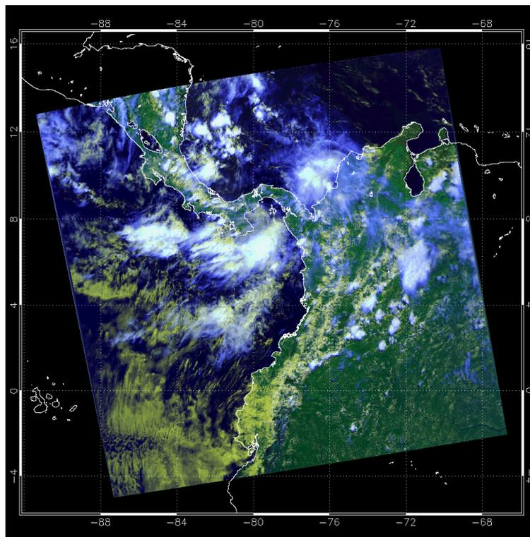
**Fig. 2.** The false-color image (Red: reflectance in  $0.65\text{-}\mu\text{m}$  band; Green: reflectance in  $0.86\text{-}\mu\text{m}$  band; Blue: Brightness temperature of  $11\text{-}\mu\text{m}$  band after gray flopped) of the Aqua MODIS granule selected for comparison. In the image, ocean is dark, land is green, low level clouds appear yellowish and high level clouds are white or light blue.
