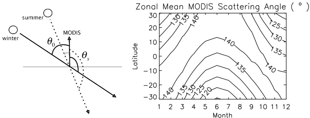
**Fig. 9.** (a) Schematic illustration of the seasonal dependence of solar zenith angle  $\theta_0$  and MODIS scattering angle  $\theta_s$ . (b) Zonal mean  $\theta_s$  as functions of latitude and month.
