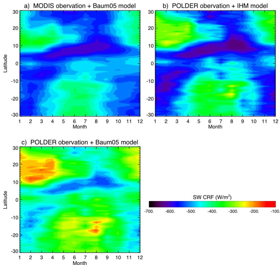
**Fig. 6.** Three sets of ice cloud shortwave CRF. **(a)** is derived from MODIS ice cloud  $\tau$  retrieval in Fig. 5a using the Baum05 model to specify the radiative properties of ice particles. **(b)** from POLDER retrieval in Fig. 5b using the IHM model. **(c)** same as (b) except that the Baum05 model is used.
