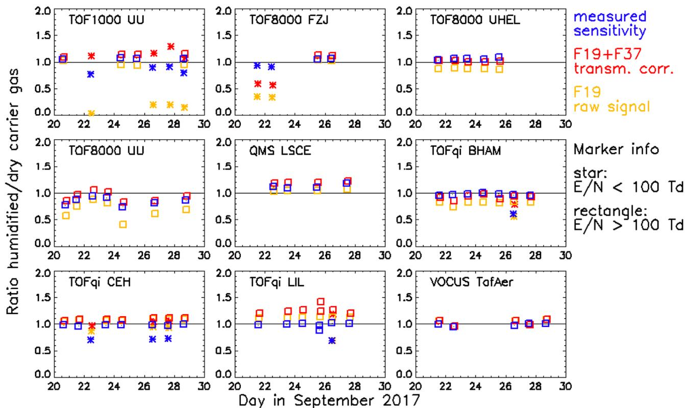
**Figure 8.** Comparison of gas standard injections using humidified and dry carrier gas. The ratios obtained for humidified versus dry injections are shown for (i) the mean measured sensitivity of a core set of compounds (blue), (ii) the transmission corrected primary ion signal (red), and (iii) the raw  $\text{H}_3\text{O}^+$  signal (yellow). The symbols separate measurements done at  $E/N$  levels above (rectangles) or below (stars) 100 Td.
