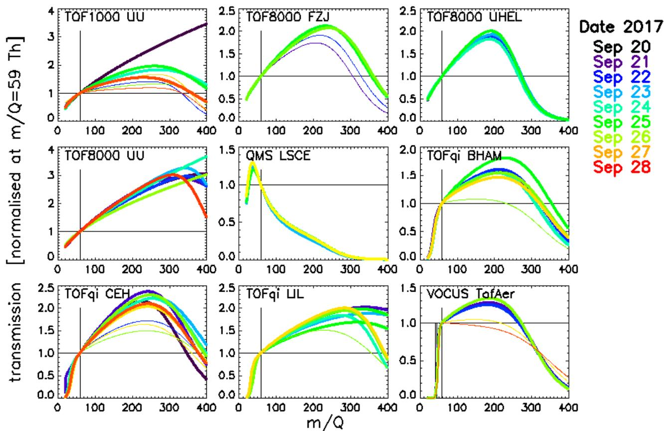
**Figure 3.** Retrieved transmission for all PTR-MS instruments (except the PTR3 instrument). Thin lines represent measurements at  $E/N$  below 150 Td, and 100 Td for the Vocus, and all other instruments, respectively. The colours indicate the date of the measurements.
