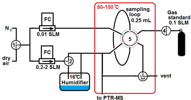
**Figure 1:** Schematic of the semi-automated calibration unit. Manual 3-way valves allow selection of dry air or nitrogen as carrier gas (valve 1), dry or humidified carrier gas (valve 2), and sample loop injections or dynamic mixing of carrier gas and gas standard (valve 3). Valve 4 (PFA-solenoid) and valve 5 (Valco 6-port with Restek sulfinert coating) are controlled to
