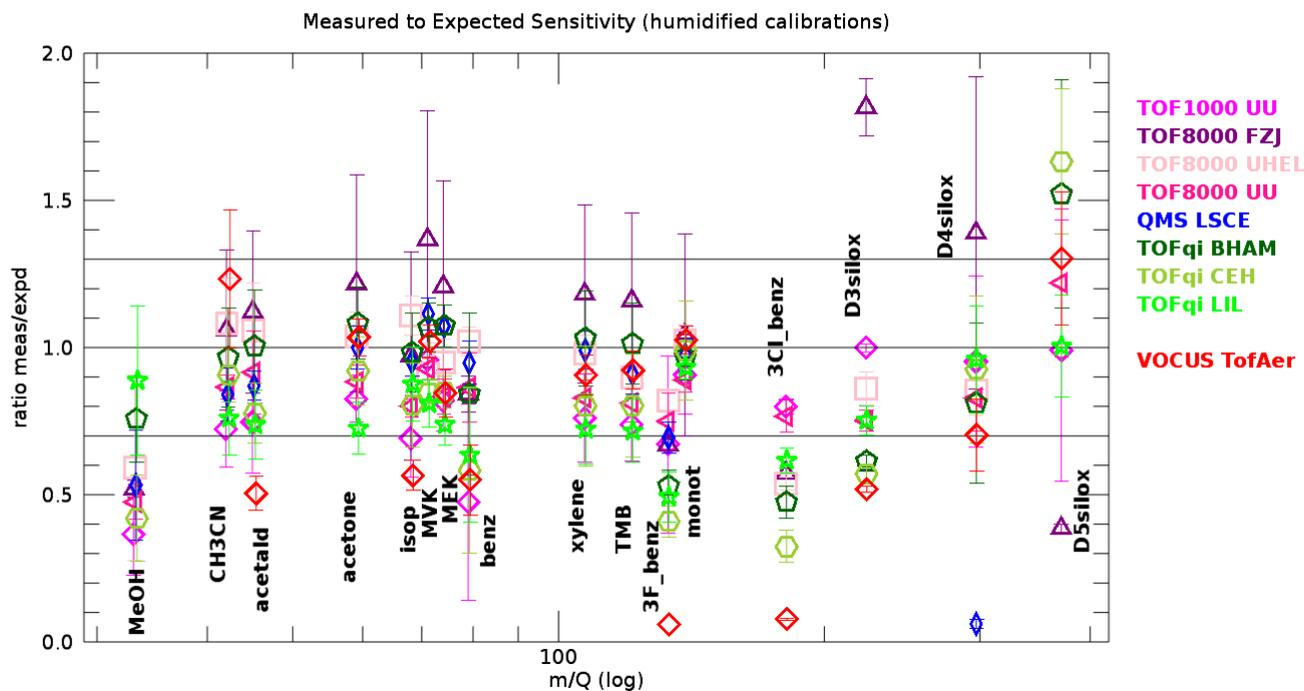
**Figure 7.** Measured versus expected sensitivities retrieved from humidified injections for all compounds in the gas standard and all PTR-MS instruments. The error bars represent the standard deviation of all gas standard injections with humidified N<sub>2</sub> or air as carrier gas. Compounds as in Figure 4.
