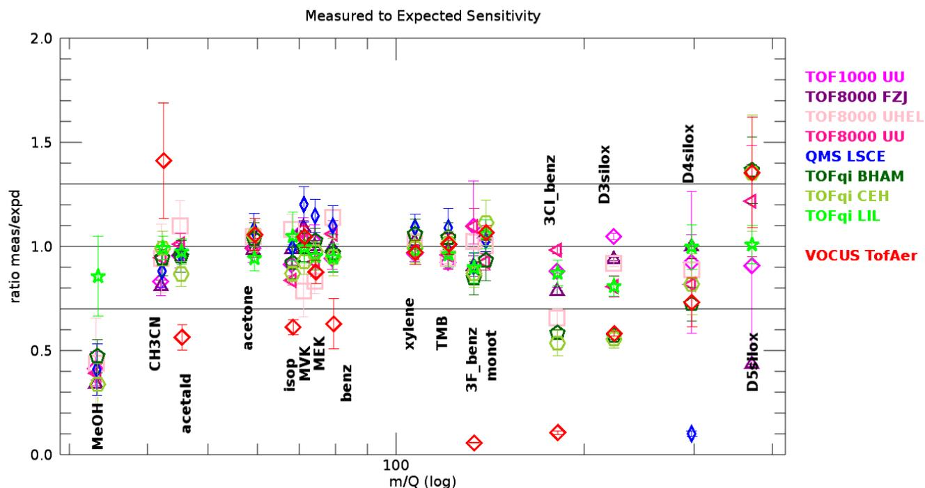
**Figure 5.** The ratio between measured and expected sensitivities as retrieved from dry injections that were not used for transmission retrievals. The data for most compounds and most instruments are well within +/- 30%. The error bars represent the standard deviation of all gas standard injections with dry N<sub>2</sub> or air as carrier gas, except those that were used to calculate the transmission. Compounds as in Figure 4.
