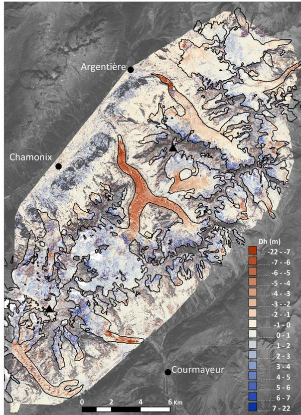
**Figure 5.** Elevation differences between the Pléiades DEMs of 21 August 2012 and 20 September 2013 over the Mont-Blanc area. The outlines of glaciers in August 2003 are shown as black lines. The southernmost triangle locates the summit of Mont Blanc (4810 m a.s.l.) and the northernmost triangle the summit of Aiguille Verte (4122 m a.s.l.). Background: SPOT5 image acquired 19 August 2003 (© CNES 2003, Distribution Spot Image).
