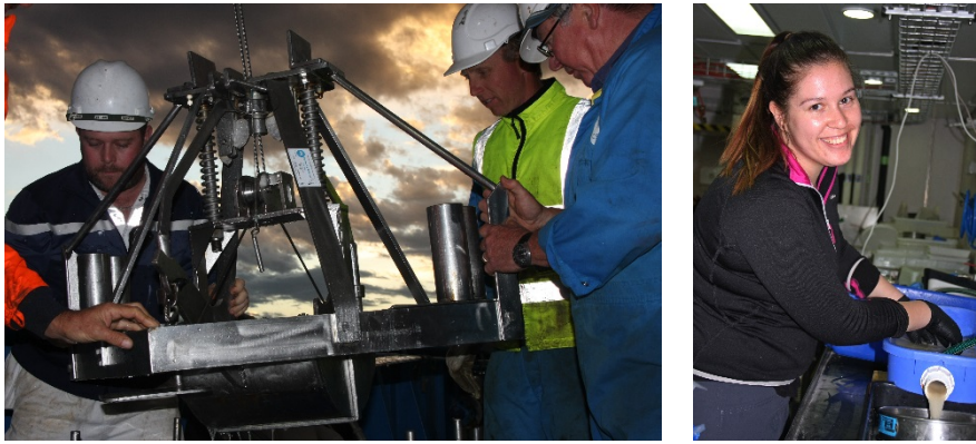
Figure 14: Deploying the Smith-McIntyre grab; sediment sample being elutriated.
