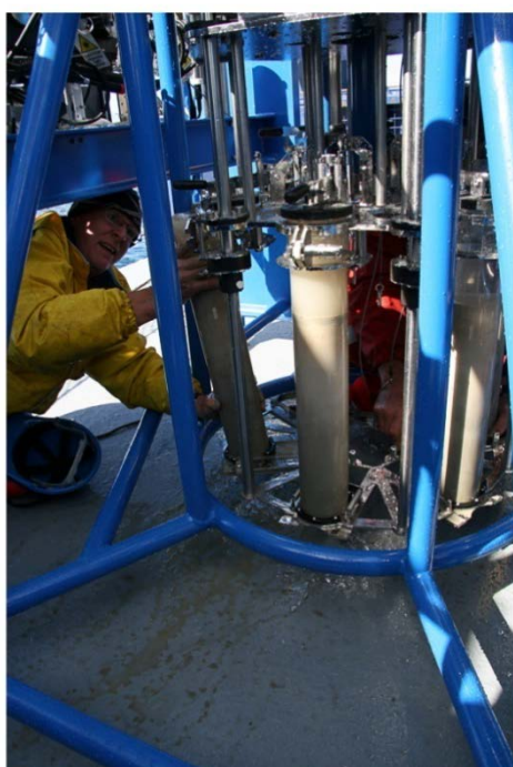
Figure 13: Sediment cores being removed from the ICP, and as recorded photographically in the core extruder.
