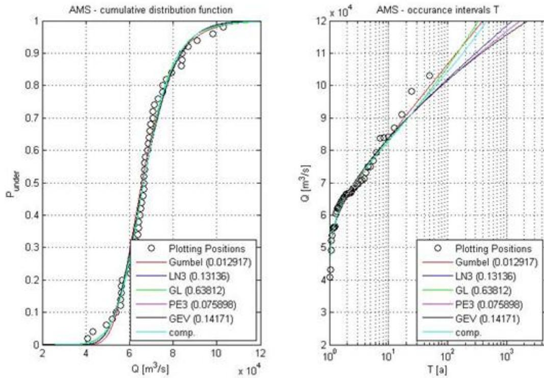
Figure 1. Different distribution functions fitted to the annual maximum flood series 1956-2004 of the gauge Bahadurabad, Brahmaputra River. **a)** cumulative probability ( $P_{\text{under}}$ ) versus computed discharge ( $Q$ ) of fitted distributions; **b)** computed discharge ( $Q$ ) of fitted distributions versus return period ( $T$ ). Comp. refers composite distribution
