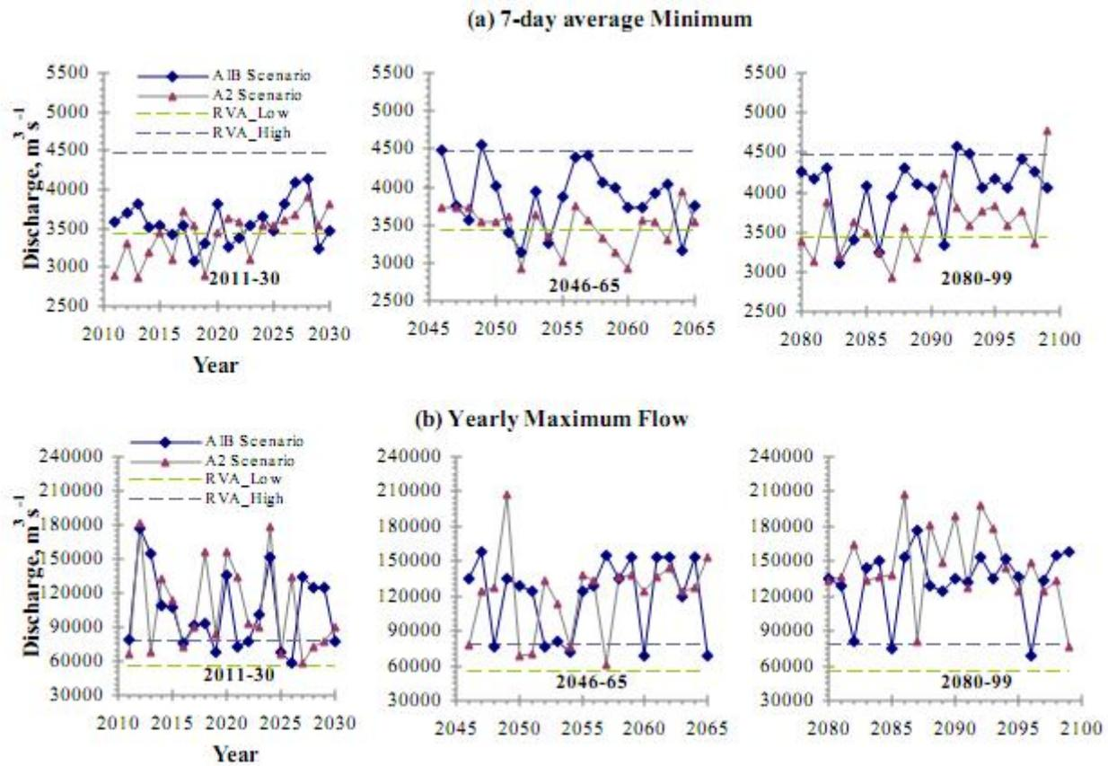
Figure 2. Investigation of thresholds values for future A1B and A2 Scenarios of **a)** 7-day average yearly minimum flow; **b)** yearly maximum flow. RVA\_Low denotes minimum threshold limit whereas, RVA\_High refers maximum threshold
