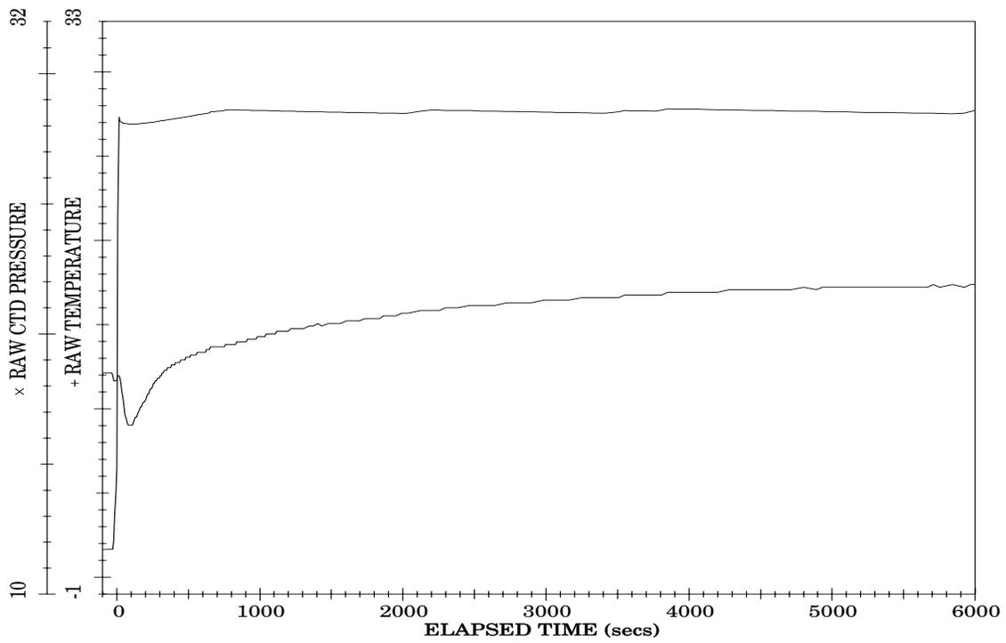
Figure 2b: CTD #1 Cold-to-Warm Thermal Shock Data
