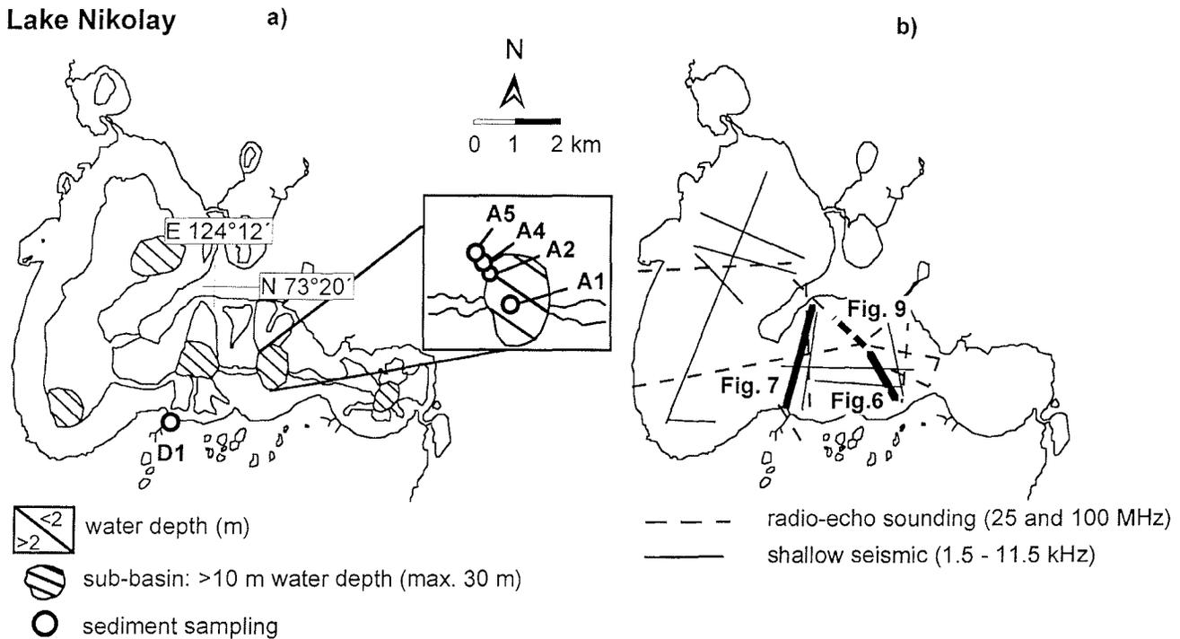
**Fig. 3:** Lake Nikolay: (a) bathymetry and sediment sampling sites (box). Sub-basins and shallow margins are delineated as measured by a portable infrared sounder aboard a rubber boat and with the aid of aerial photography. (b) shows the positions of geophysical profiles. Profiles described in the text are shown in bold lines; Figure numbers are indicated.
