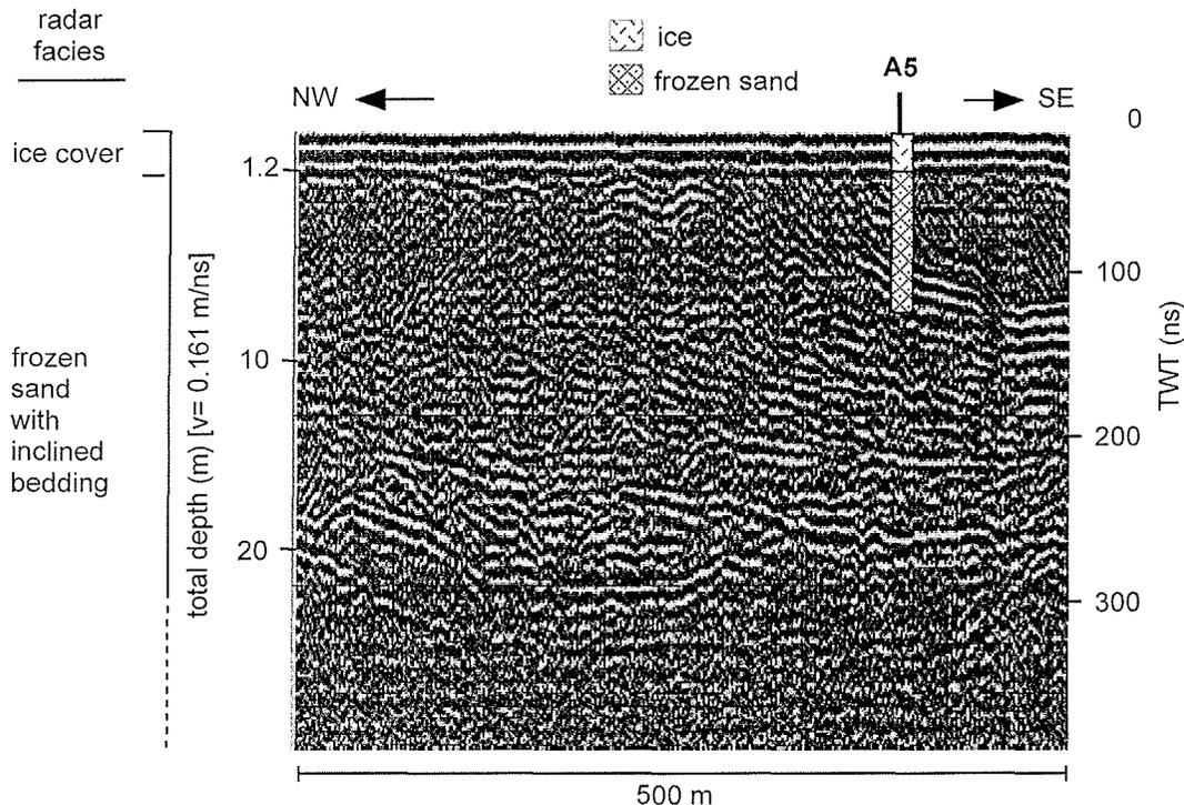
Fig. 9: Radar profile obtained with the 100 MHz antenna pair and drilling results of core A5.
