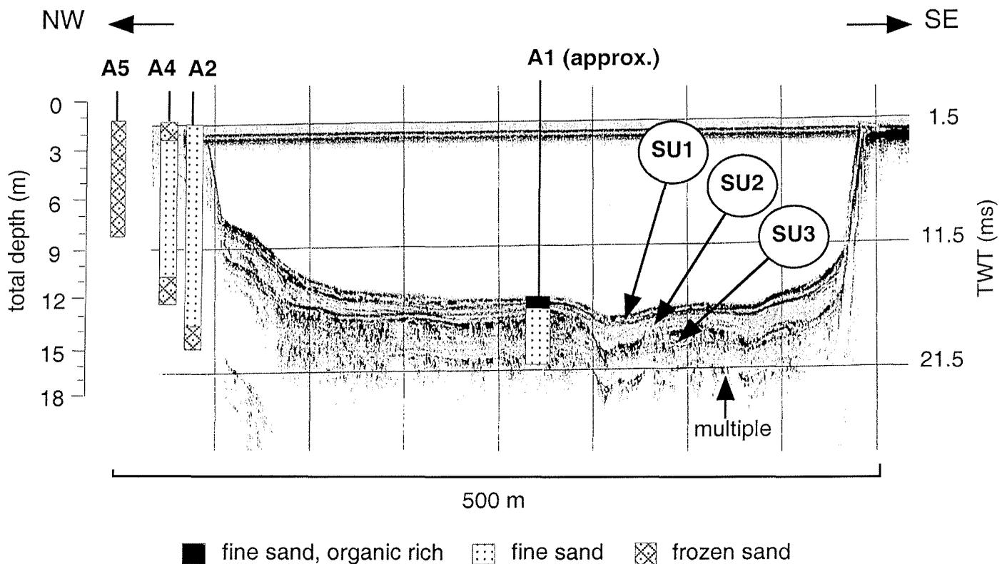
Fig. 6: Shallow seismic profile illustrating the acoustic stratigraphy of the studied basin sediments (VE : ~1:5). For interpretations of the seismic units 1 through 3 (SU 1-3) see the text. Approximate locations of sampling sites A1, A2, A4 and A5 are indicated.
