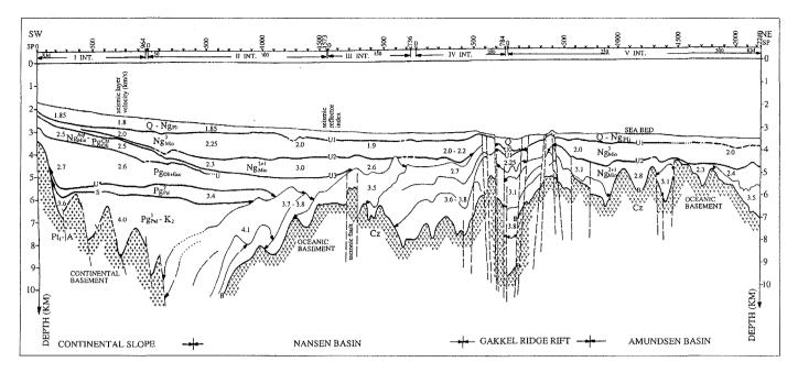
Fig. 4: Seismic line 90700. Depth section. According to the data acquisition the whole transect consists of five parts with shot point sequences: I INT, II INT, III INT, IV INT, V INT, V INT, On top the shot points (SP) and their numbers as well as the horizontal scale in kilometers. The seismic units accordingly to Figure 3 are included as well as their seismic velocities in km/s. Assumed stratigraphic ages based on these studies are indicated.
