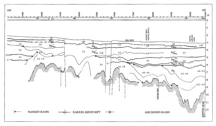
Fig. 6: Fragment of the seismic line 90702. Depth section. According to the data acquisition the whole transect consists of three parts with shot point sequences: I INT, III INT, On top the shot points (SP) and their numbers as well as the horizontal scale in kilometers. Seismic units according to Figure 3 are included as well as seismic velocities in km/s. Assumed stratigraphic ages based on these studies are indicated.
