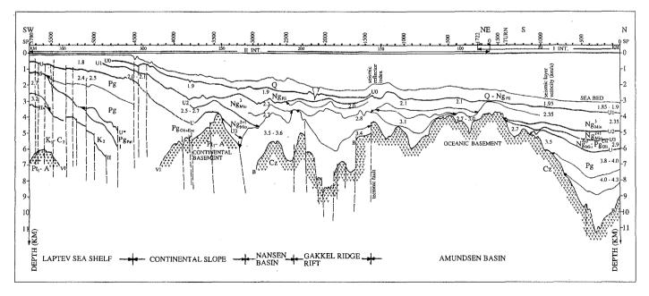
Fig. 7: Seismic line 90704. Depth section. According to the data acquisition the whole transect consists of two parts with shot point sequences: I INT, II INT. On top the shot points (SP) and their numbers as well as the horizontal scale in kilometers. Seismic units according to Figure 3 are included as well as seismic velocities in km/s. Assumed stratigraphic ages based on these studies are indicated.
