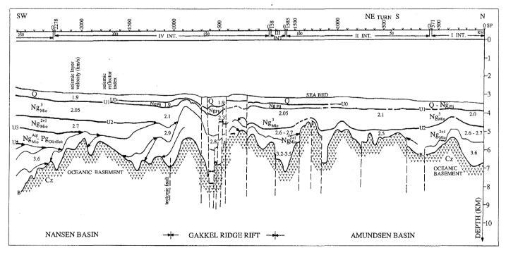
Fig. 5: Fragment of the seismic line 90701. Depth section. According to the data acquisition the whole transect consists of five parts with shot point sequences: I INT, II INT, III INT, IV INT, V INT. On top the shot points (SP) and their numbers as well as the horizontal scale in kilometers. Seismic units according to Figure 3 are included as well as seismic velocities in km/s. Assumed stratigraphic ages based on these studies are indicated.
