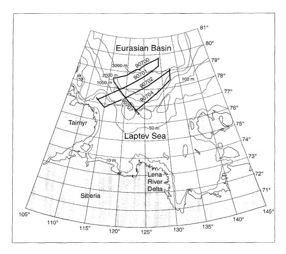
Fig. 1: Bathymetric chart of the Laptev Sea and adjacent part of the Eurasian Basin and location of the MAGE seismic lines 90700, 90701, 90702, 90704 and 90707. Bathymetric contours are given in metres. Map produced with GMT software (WESSEL & SMITH 1995).
