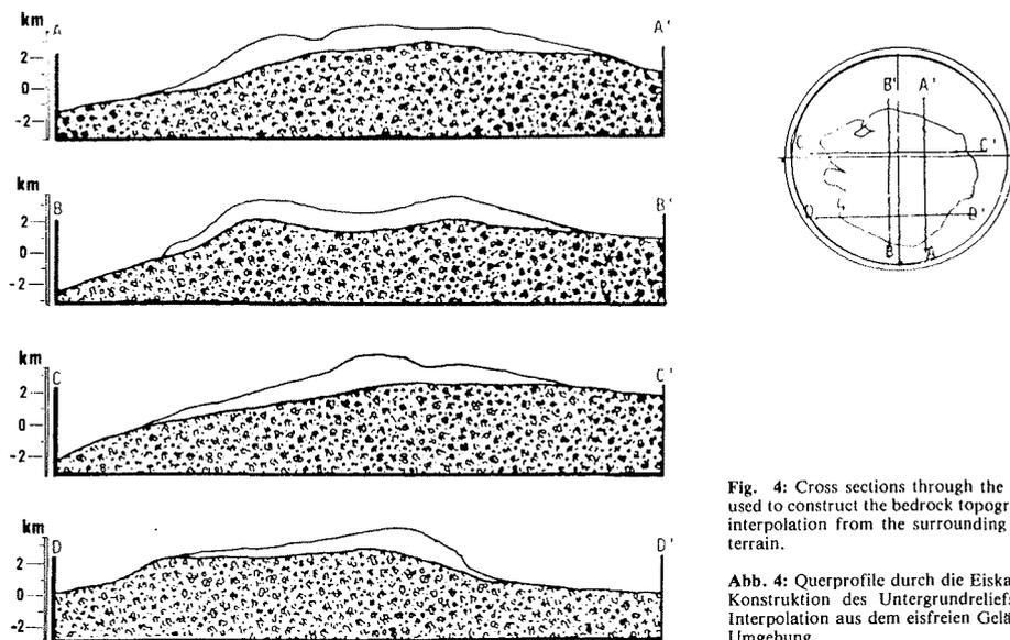
Fig. 4: Cross sections through the ice cap, used to construct the bedrock topography by interpolation from the surrounding ice-free terrain.
