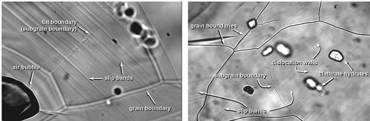
Figure 7: Microstructural features of Antarctic ice revealed by the method of microstructure mapping. Left: Slip bands, air bubbles and a subgrain boundary in a sample from 610 m depth, EPICA-Dome C deep ice core (from [156], with modifications). Right: Diverse microstructural features in a sample from 1320 m depth, EPICA-DML deep ice core (from [92], with modifications). The width of each image is 700  $\mu\text{m}$ .
