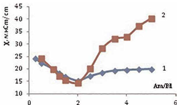
**Figure 5.** Electrical conductivity of  $1 \cdot 10^{-4}$  M aqueous solution of  $K_2[PdCl_4]$  depending on the metal/amine molar ratio with the addition of: 1-2-AP; 2-4-AP.
