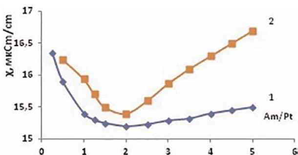
**Figure 6.** Electrical conductivity of  $1 \cdot 10^{-4}$  M aqueous solution of  $K_2[PtCl_4]$  depending on the metal/amine molar ratio with the addition of: 1-2-AP; 2-4-AP.
