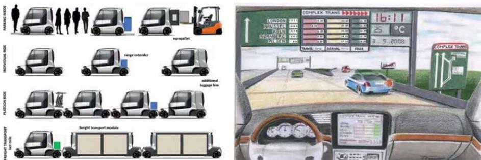
**Figure 21.** Left—parking and ride of the coupemobiles—individual or in platoon, electric or with range extender. Bottom left—Freight transport modules are also carried in vehicle platoons over distances up to 50–100 km. Right—when leaving a large city, the driver of the coupemobile has the choice between road and rail.
