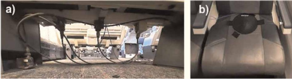
**Figure 3.** Accelerometer positioning: (a) seat frame and floor accelerometers, (b) seat surface pad.
