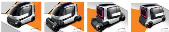
**Figure 7.** Coupemobile, a passenger e-car of the ComplexTrans system for the comfortable transport of five adults and their luggage. Retractable axles, from the back swappable battery, roof grip points and couplers give these cars a whole new range of possibilities, an “unlimited” range and a widely acceptable price.
