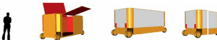
**Figure 8.** Long and short freight transport module for transporting goods in ComplexTrans mixed trains. It has its own electric drive, is transported to the end users by road platoons with a guiding vehicle, and can be remotely controlled for local manipulation.
