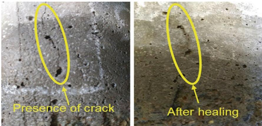
Fig. 7.8 Combined bacterial concrete before and after healing
