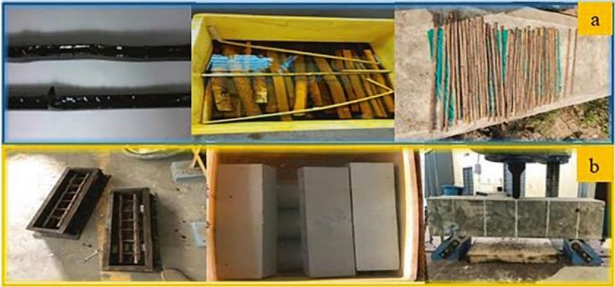
**Fig. 3.2** Bamboo-reinforced concrete beams: (a) bamboo treatment, (b) casting and testing of bamboo-reinforced concrete beams
