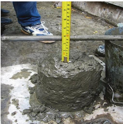
was good. Furthermore, the amount of water required was smaller than in the other three scenarios, which could result in a sustainable and cost-effective outcome. The lower the slump, the harder and less workable the concrete would be, but the hardness should not be much less as it would be difficult to construct. Blend 4 had greater strength and durability than other cases, as it is commonly known that the higher the slump, the lower the strength and durability.
