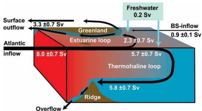
Figure 12: Overall budget for the AM-exchanges where the circulation within the AM is simplified into two loops: a thermohaline loop converting Atlantic inflow and freshwater into overflow, and an estuarine loop converting all three types of AM-import into surface outflow.
