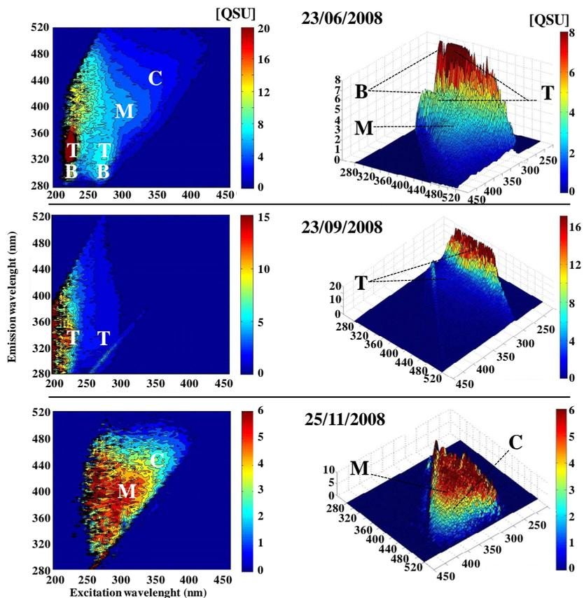
**Fig. 5.** 2-D (left panel) and 3-D (right panel) EEM contour plots of CDOM (in QSU) acquired at SOFCOM station at 5 m depth on 23 June 2008, 23 September 2008 and 25 November 2008. These spectra illustrated the fluorophore peak positions observed during this study. 3-D spectra are shown from reverse side to facilitate viewing of humic-like peak (peak C).
