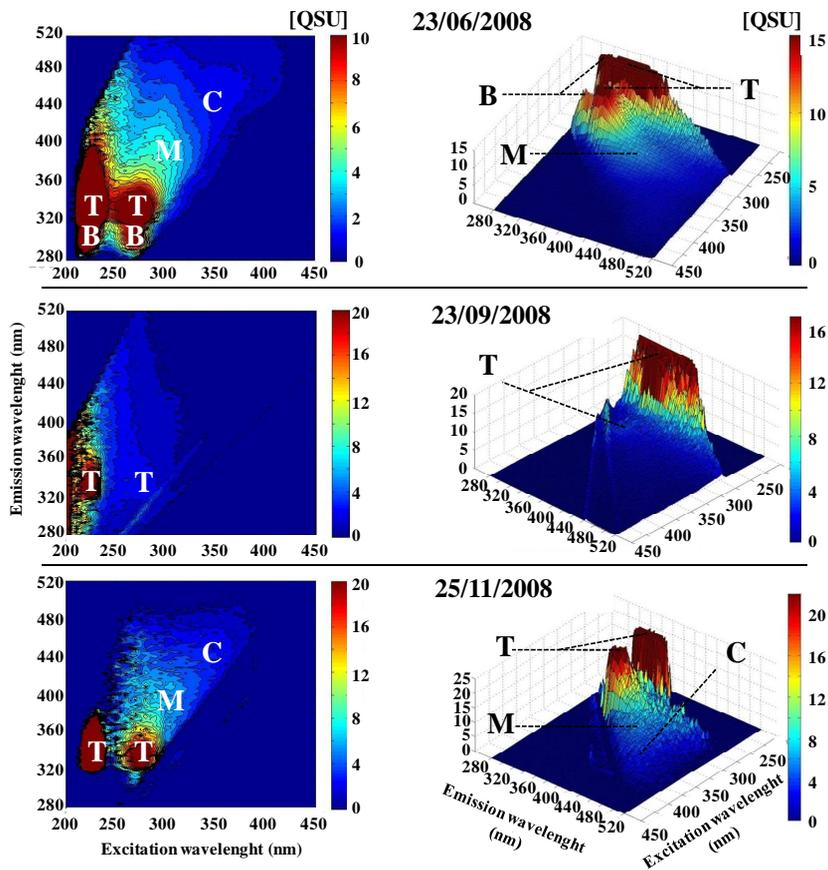
**Fig. 4.** 2-D (left panel) and 3-D (right panel) EEM contour plots of CDOM (in QSU) acquired at SOFCOM station at 2 m depth on 23 June 2008, 23 September 2008 and 25 November 2008. These spectra illustrated the fluorophore peak positions observed during this study. 3-D spectra are shown from reverse side to facilitate viewing of humic-like peak (peak C).
