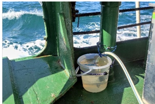
Fig. 3.2: continuous sampling of dissolved phycotoxins by SPATT
