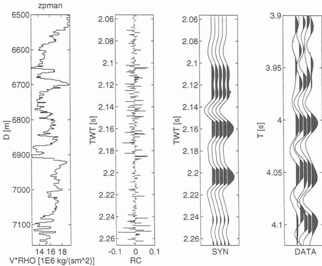
Abb. 7 : Comparison between Synthetic Seismogram and INSTRUCT Reflection Data
