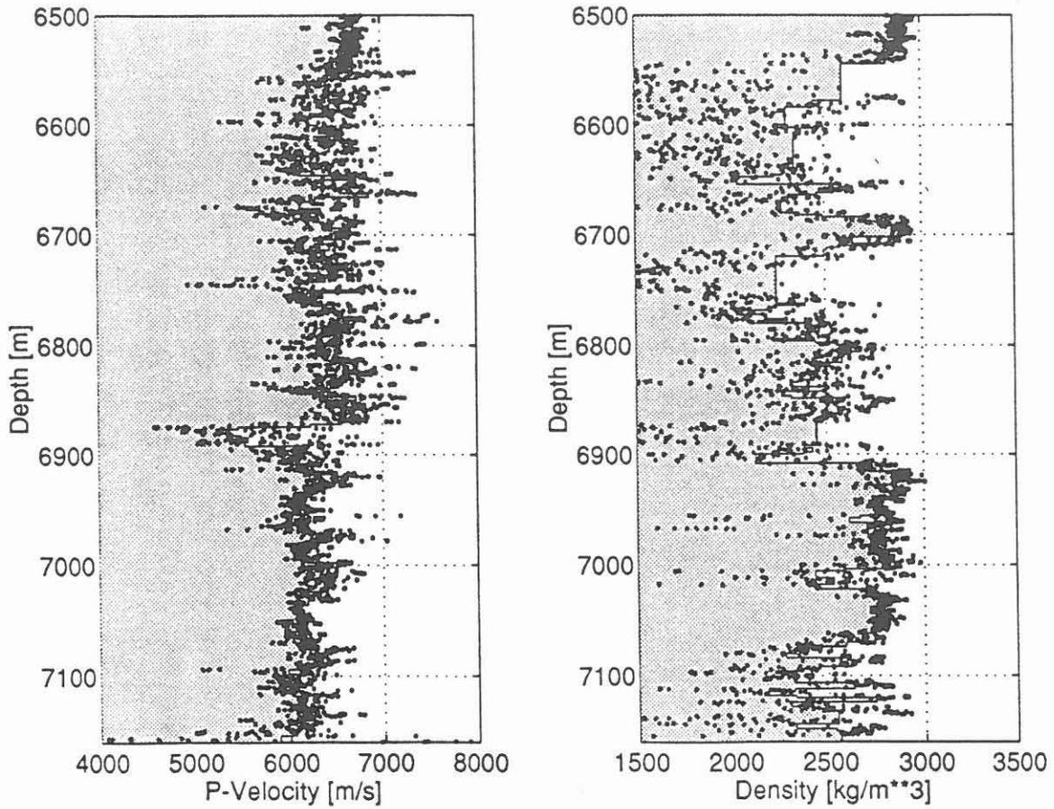
Abb. 2 : Sonic Log and Density Log within Depth-Range of SE-1 Reflector (KTB)
