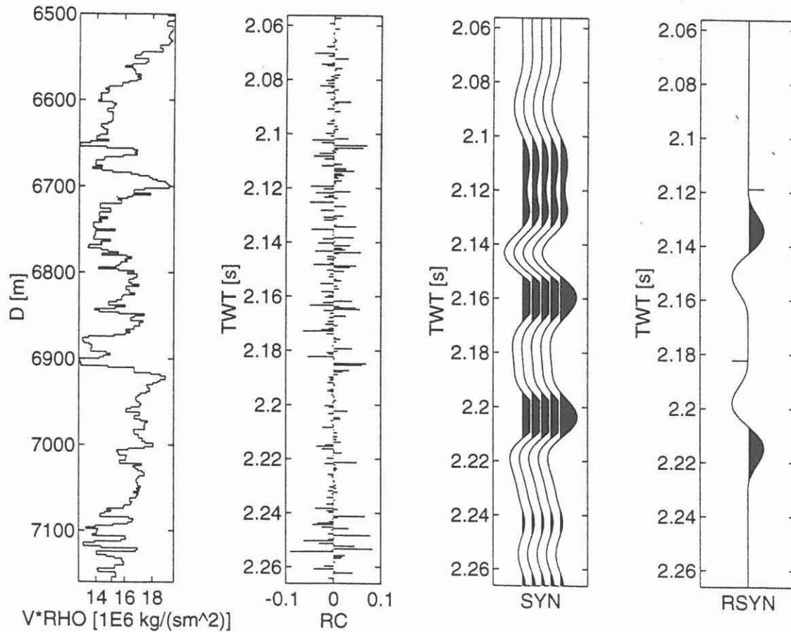
Abb. 3 : Impedance, Reflectivity and Synthetic Seismogram for SE-1 Reflector (KTB)
