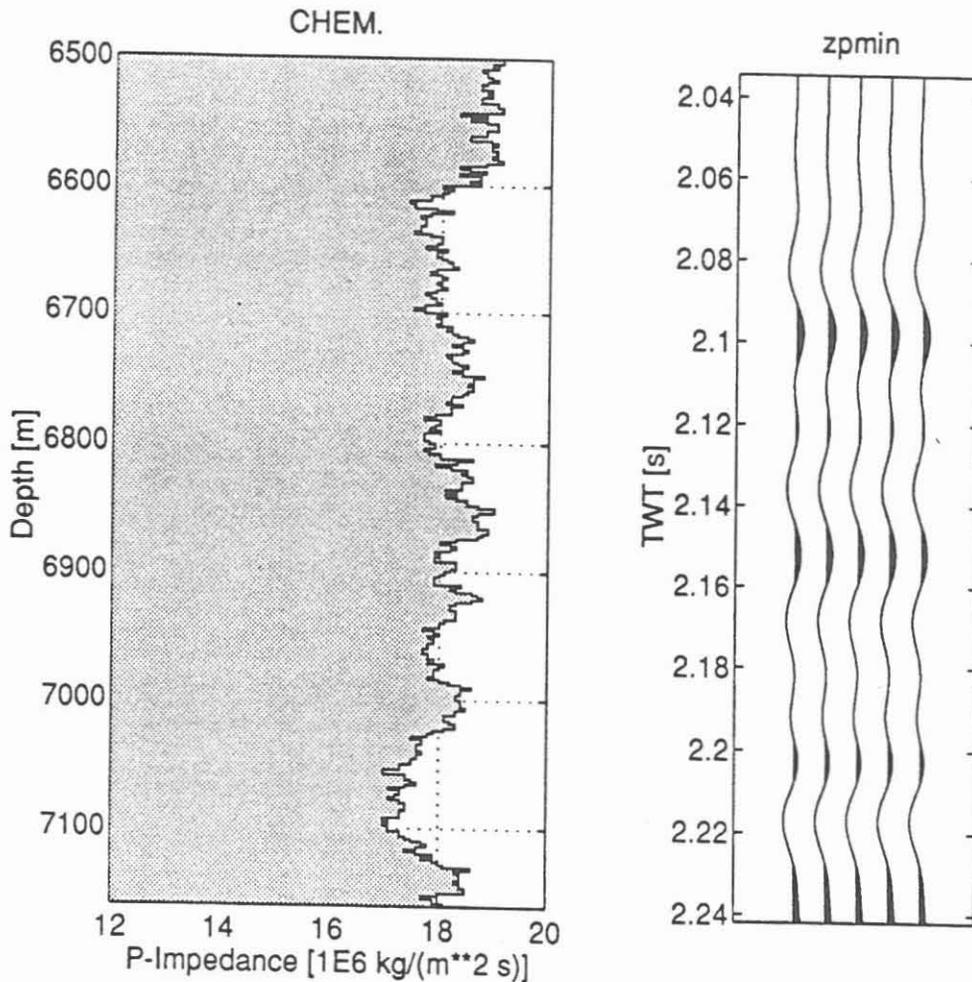
Abb. 4 : Impedance log (left) calculated from Mineral Composition of Cuttings and Corresponding Synthetic Seismogram
