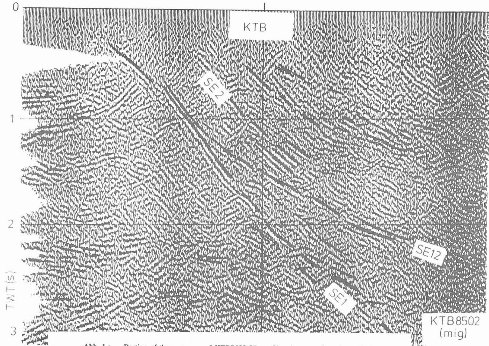
Abb. 1 : Portion of the re-processed KTB8502 2D-profile, phase consistently stacked, migrated and coherency filtered. From DPC, Clausthal.
