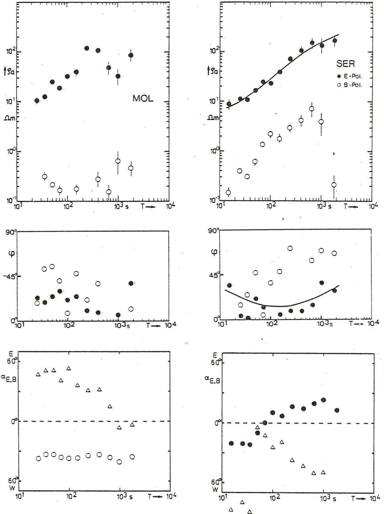
**Fig. 3b:** Apparent resistivities, phase differences and azimuths at the stations MOL and SER. The site MOL has been measured in 1979 (Haak & Schwarz, 1981). The consistency between  $\rho_a$  and phase at the site SER has been proved by 1D-modelling: the drawn curves result from a two-layered-model (not shown here).
