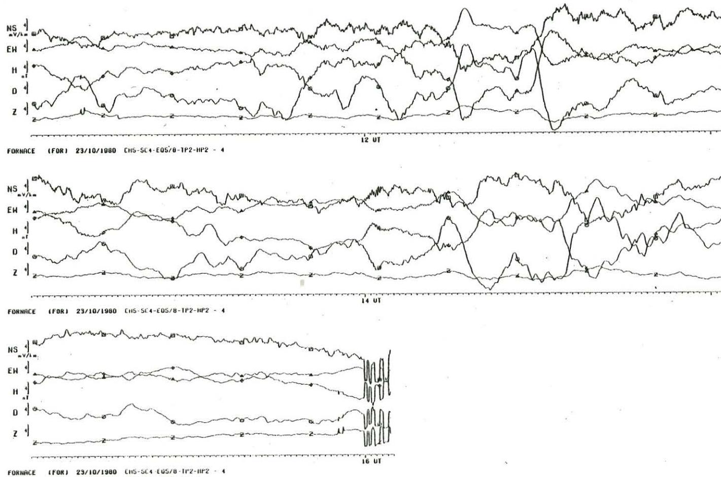
Fig. 2: Recording sample of the time varying electric and magnetic field at the station FOR. The upper two traces represent the two horizontal components of the electric field, the lower three traces the components of the magnetic field.
