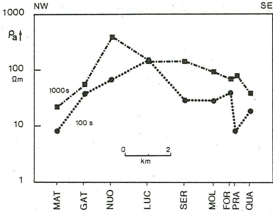
Fig. 5: Variation of the apparent resistivities on a profile parallel to the Travale Graben, running out of the known geothermal field towards NW.
