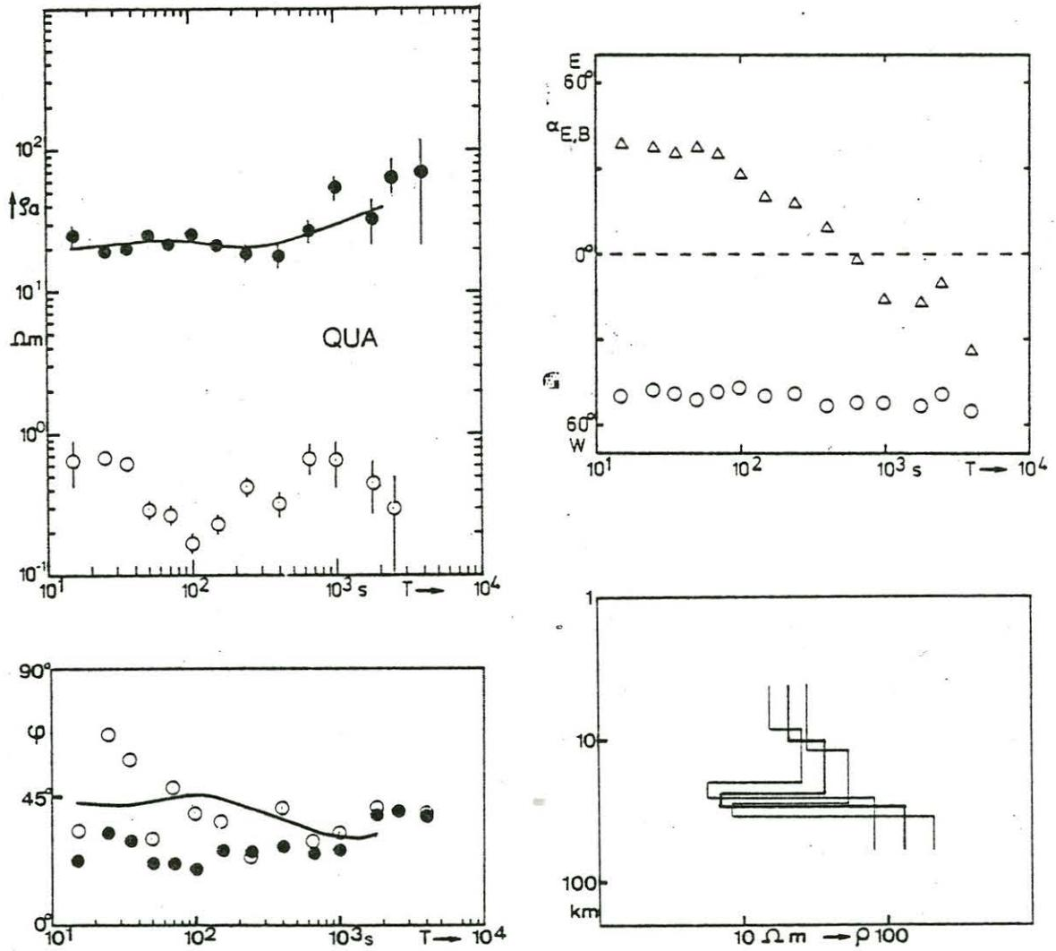
Fig. 3: Uppermost panel on the left the apparent resistivity as function of period, calculated in the maximum-minimum-coordinate system. The black dots represent the E-mode, open circles represent B-mode. Below the phasedifferences between E- and B-field. Uppermost panel on the right the azimuths of both fields ( $\circ$ : rotation angle of E-field,  $\Delta$ : rotation angle of B-field), below the resistivity-models obtained by an inversion algorithm from the apparent resistivities.
