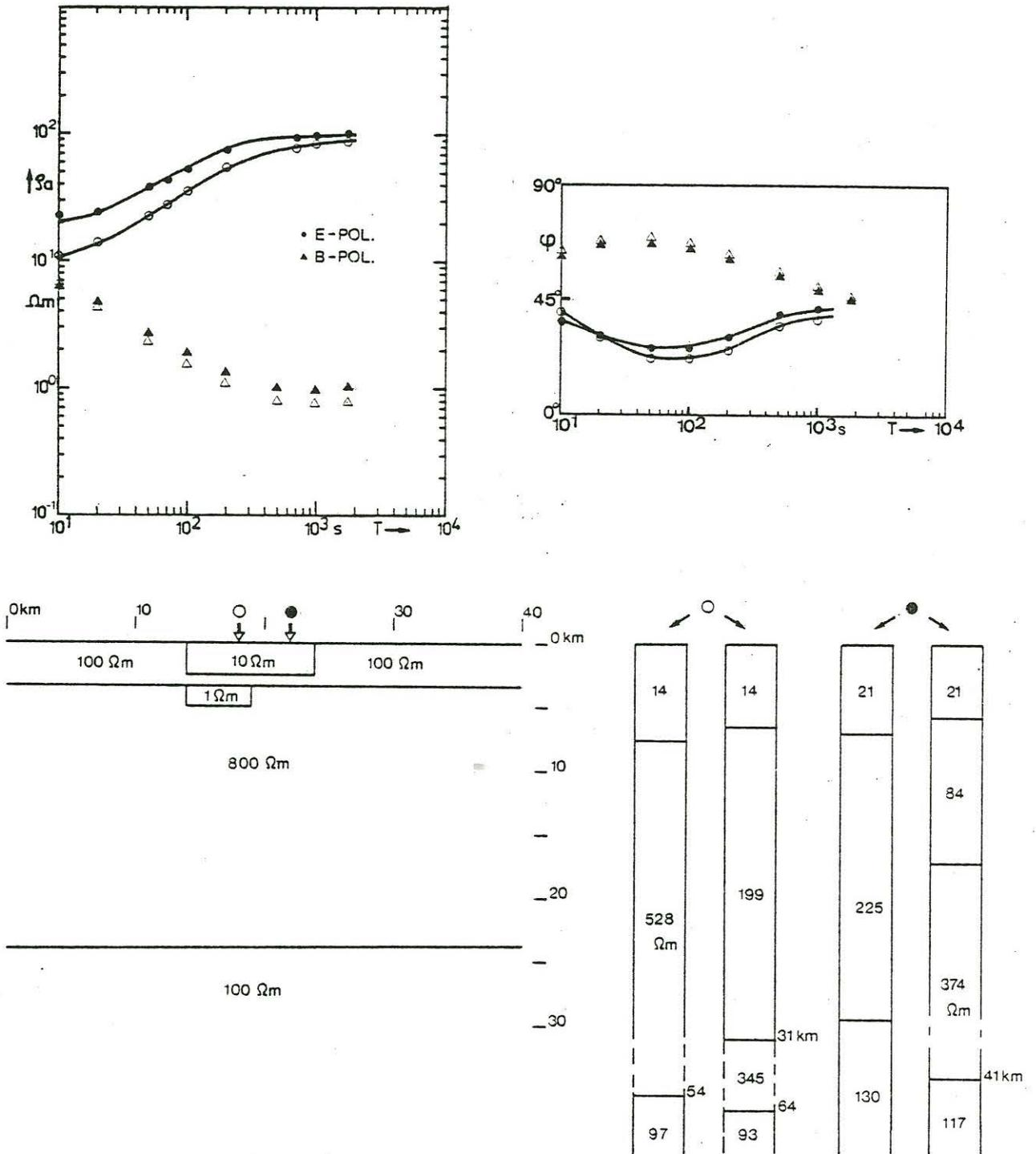
Fig. 6: Shallow graben model with corresponding apparent resistivity curves of two sites in the middle of the graben. On the right: the apparent resistivity curves were interpreted by a 1D-inversion algorithm.
