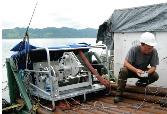
Fig. 6.6: Logging winch with 2.2 km of a 4-conductor cable
