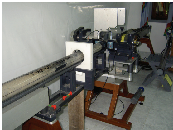
Fig. 8.1: Multi-sensor core logger in field lab
