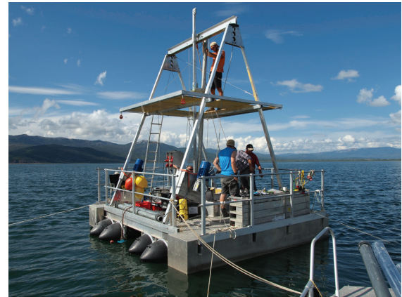
Fig. 6: Platform for taking shallow piston cores
