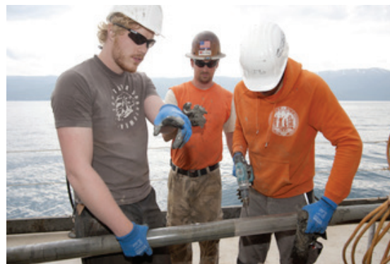
Fig. 9.7: Drill core handling on the barge. Small holes were drilled into plastic liners to prevent excessive core expansion from high gas pressure in the liner (Photo: N. Leicher).
