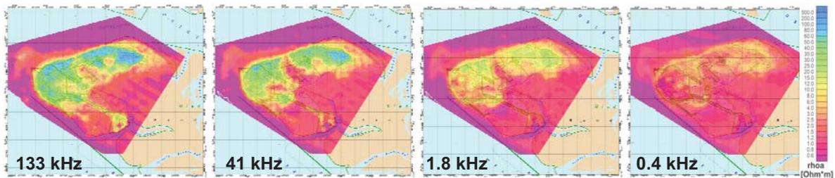
**Figure 3:** Apparent resistivity maps: The investigation depth increases with decreasing frequency. The freshwater lenses – represented by higher resistivities (green & blue) – are nearly completely penetrated by the EM fields of lowest frequency.
