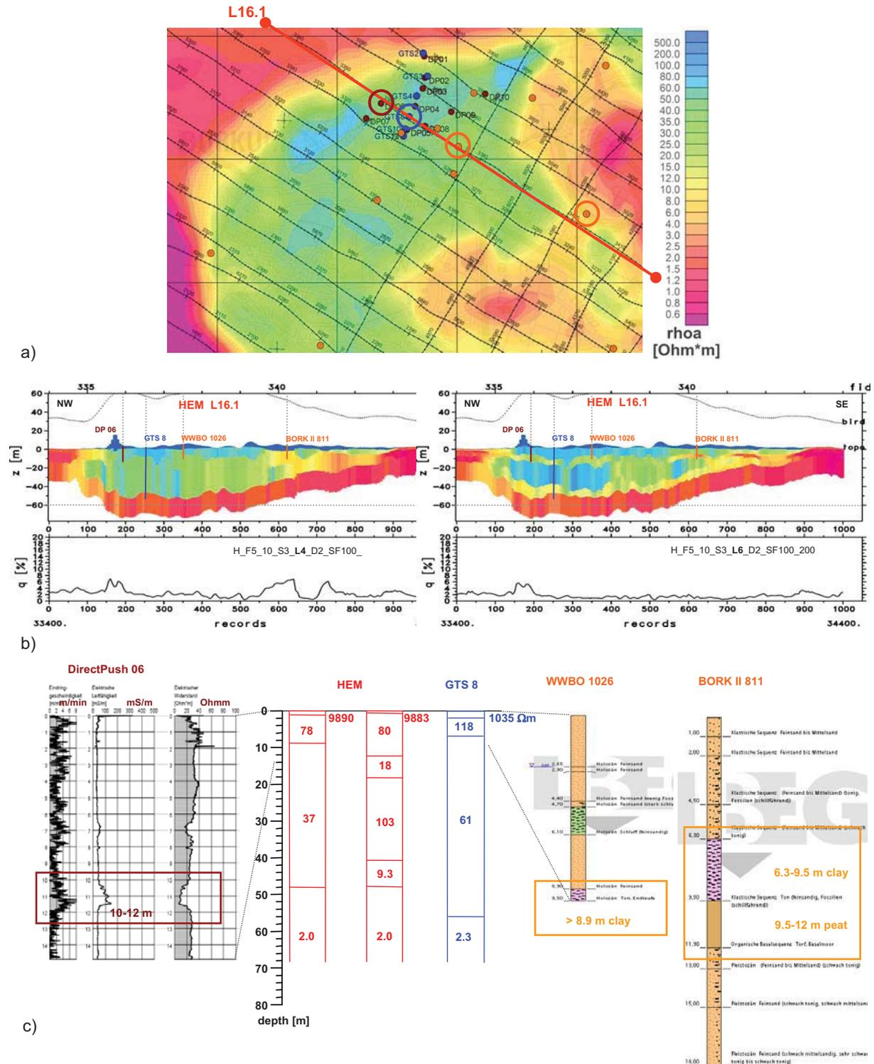
**Figure 7:** a) Apparent resistivity map (41 kHz) with the location of the vertical resistivity section L16.1, the lithological logs and the *direct-push* measurement. b) Comparison of HEM 1-D inversion results (4- and 6-layer models) along L16.1 with c) lithological logs (WWBO 1016 and BORK II 811) (LBEG), *direct-push* results (DP 06) (Winter, 2008) and DC 1-D inversion results (GTS8).
