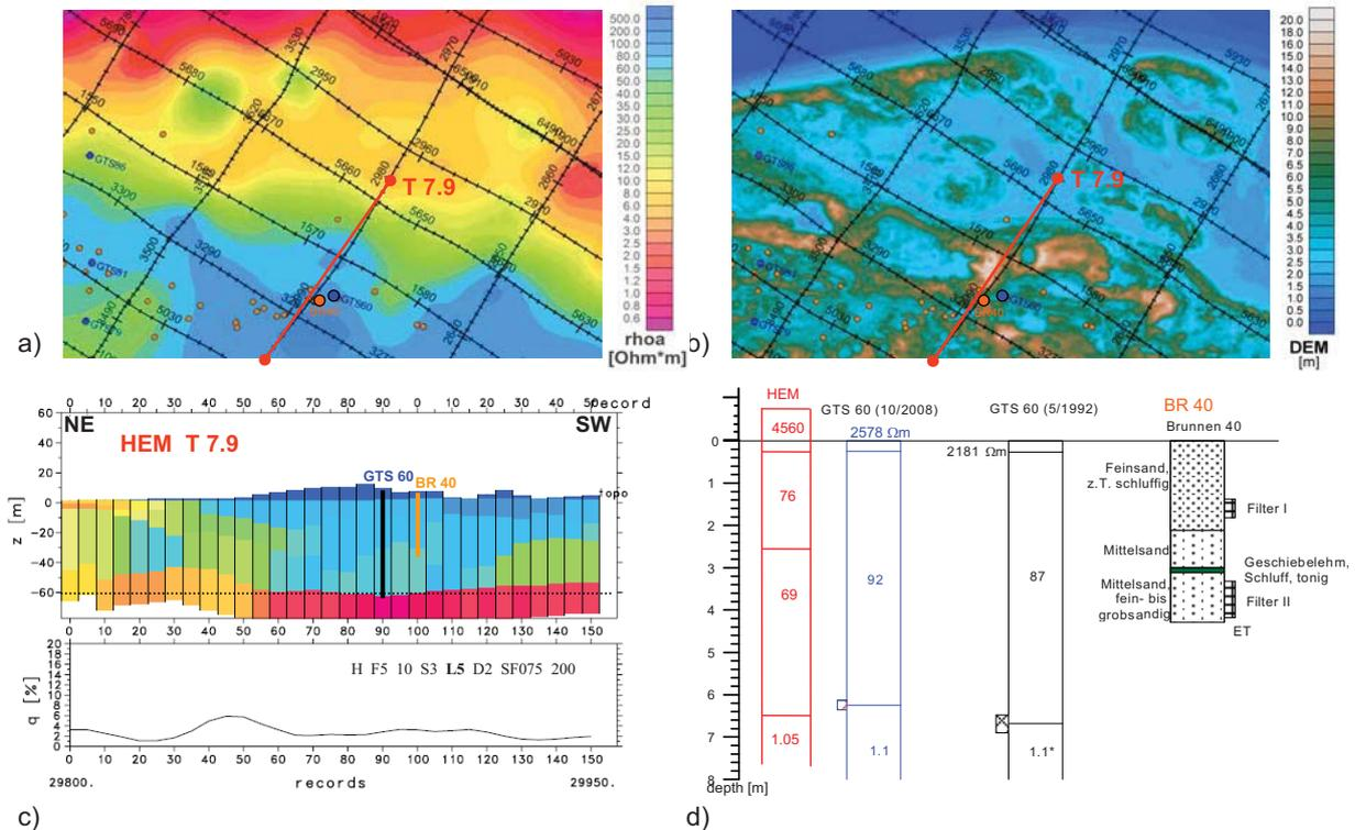
**Figure 6:** a) Resistivity map (5 mbsl) with the location of a part of flight-line T7.9 (red line), the lithological log BR40 (orange circle) and the DC site GTS 60 (blue circle). b) Digital elevation model revealed from laser scan data of *NLWKN*. c) Vertical resistivity section T7.9 as result of a 5-layer 1-D inversion (every 5<sup>th</sup> model is shown). d) Comparison of 1-D inversion results of HEM and DC reveals the freshwater/saltwater boundary at a similar depth of about 60 mbsl.
