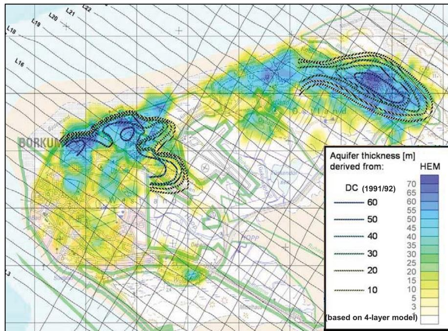
Figure 8: Aquifer thickness derived from DC and HEM.
