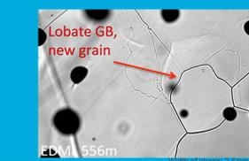
Electron Backscatter diffraction (EBSD)
