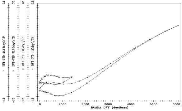
Figure 2a: CTD #2 Pre-cruise Pressure Calibration
