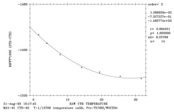
Figure 5a: CTD #2 Pre-cruise PRT-1 Temperature Calibration
