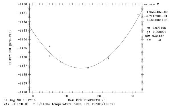
Figure 4a: CTD #1 Pre-cruise PRT-1 Temperature Calibration
