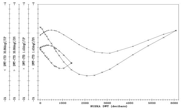
Figure 1c: CTD #1 Post-cruise Pressure Calibration
