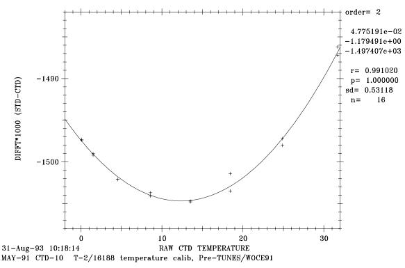
Figure 6b: CTD #10 Pre-cruise PRT-2 Temperature Calibration
