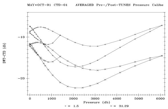
Figure 1d: CTD #1 Averaged Pre-/Post-cruise Pressure Calibration
