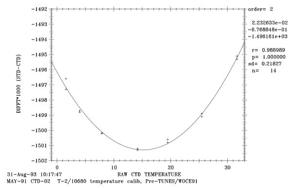
Figure 5c: CTD #2 Pre-cruise PRT-2 Temperature Calibration
