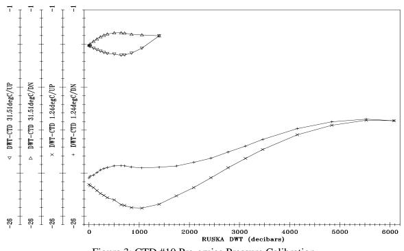
Figure 3: CTD #10 Pre-cruise Pressure Calibration
