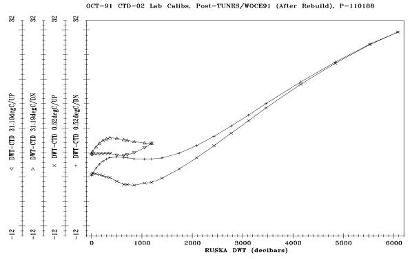
Figure 2b: CTD #2 Post-cruise Pressure Calibration
