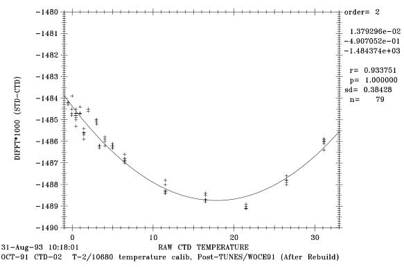
Figure 5d: CTD #2 Post-cruise PRT-2 Temperature Calibration
