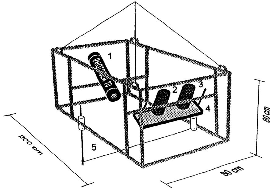
Fig. 11: Perspective view and size of the particle camera system: 1: 70 mm
