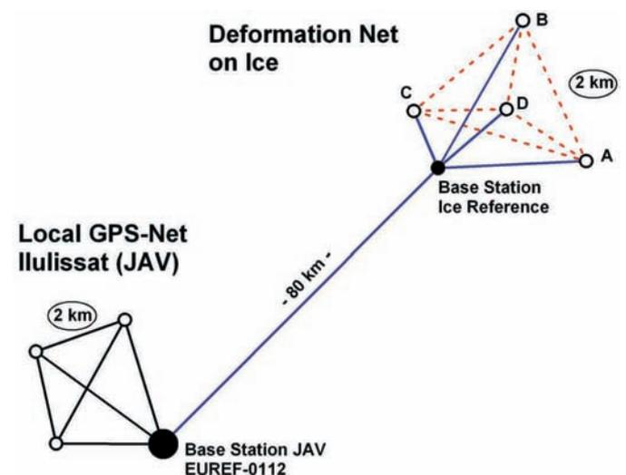
**Fig. 3:** Schematic net design of GPS measurements and deformation figure: Reference point EUREF0112 on solid rock with local backup net in Ilulissat, long baseline to the ice reference, and deformation net (triangle with central point) on the ice. Sketch without scale.
