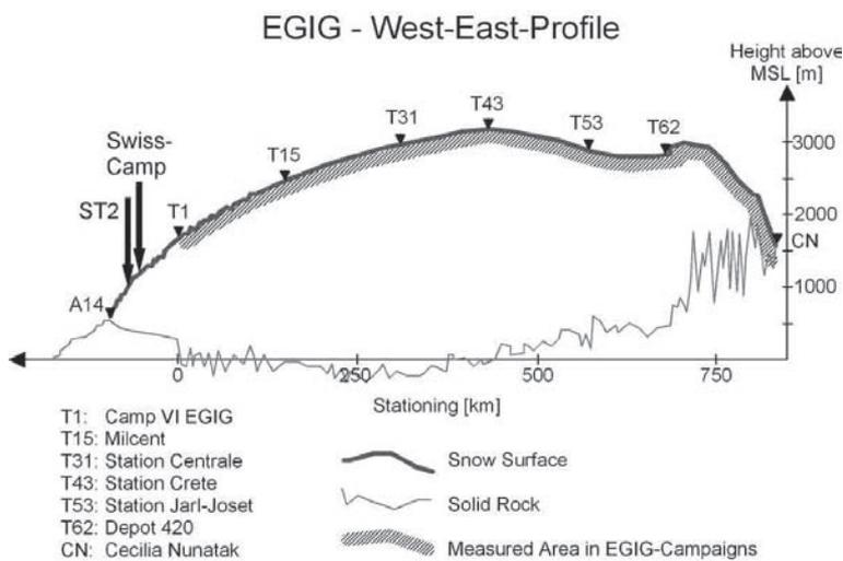
Fig. 2: Areas with repeated elevation measurements in the EGIG-line 1959, 1968, 1990/92 (see HOMANN et al. 1996) and elevation situation of recent measurements at Swiss Camp and ST2, 1991-2006.
