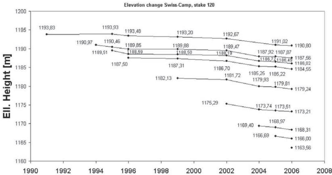
**Fig. 5:** Heights of stake 120, all reconstructed previous positions re-measured in all subsequent campaigns. All measurements were performed in summer.
