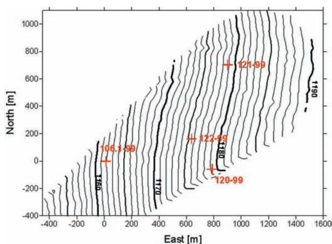
**Fig. 4:** Contour lines from digital elevation model (2006) at Swiss Camp with stake positions in 1999 (mean epoch, local coordinate system, origin = point 106.1-99).
