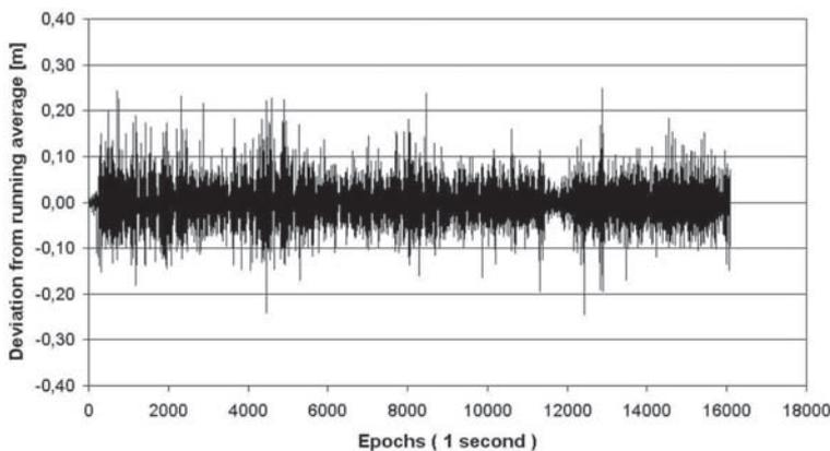
**Fig. 12:** Height deviations in kinematical GPS profiling: Single epochs minus running average. 16000 seconds corresponding to about 4.5 hours, with approximately 8 km profile measurement.
