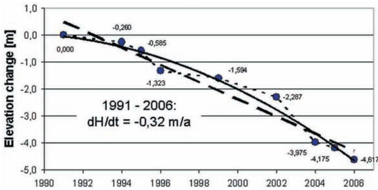
**Fig. 6:** Accumulated elevation change of ice horizon at Swiss Camp 1991-2006. Changes between campaigns = thin dashed line; linear trend = bold dashed straight line; adjusted curve second order = solid line.
