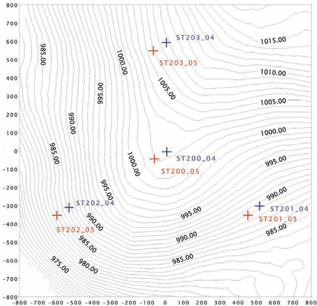
**Fig. 10:** ST2: Contour lines, derived from a digital terrain model, displacement of stakes within one year, positions 2004 (blue) and 2005 (red).
