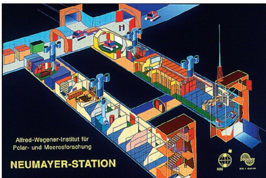
**Fig. 12:** Schematic diagram of Neumayer Station II (NM-II) showing the station design below the ice (not showing the vehicle garage), (D. Enns / Polarmar)
