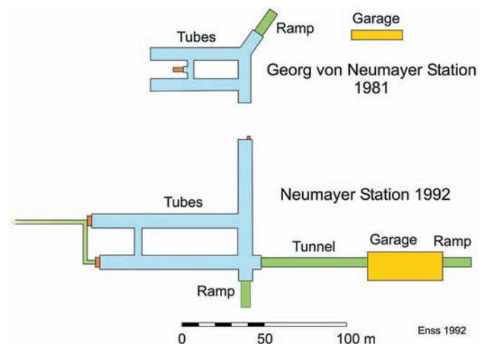
Fig. 10: Schematic diagram showing proportions of the two stations Georg von Neumayer (GvN) constructed in 1981 and its successor Neumayer Station II (NM-II) constructed in 1992 (D. Enss / Polarmar).
