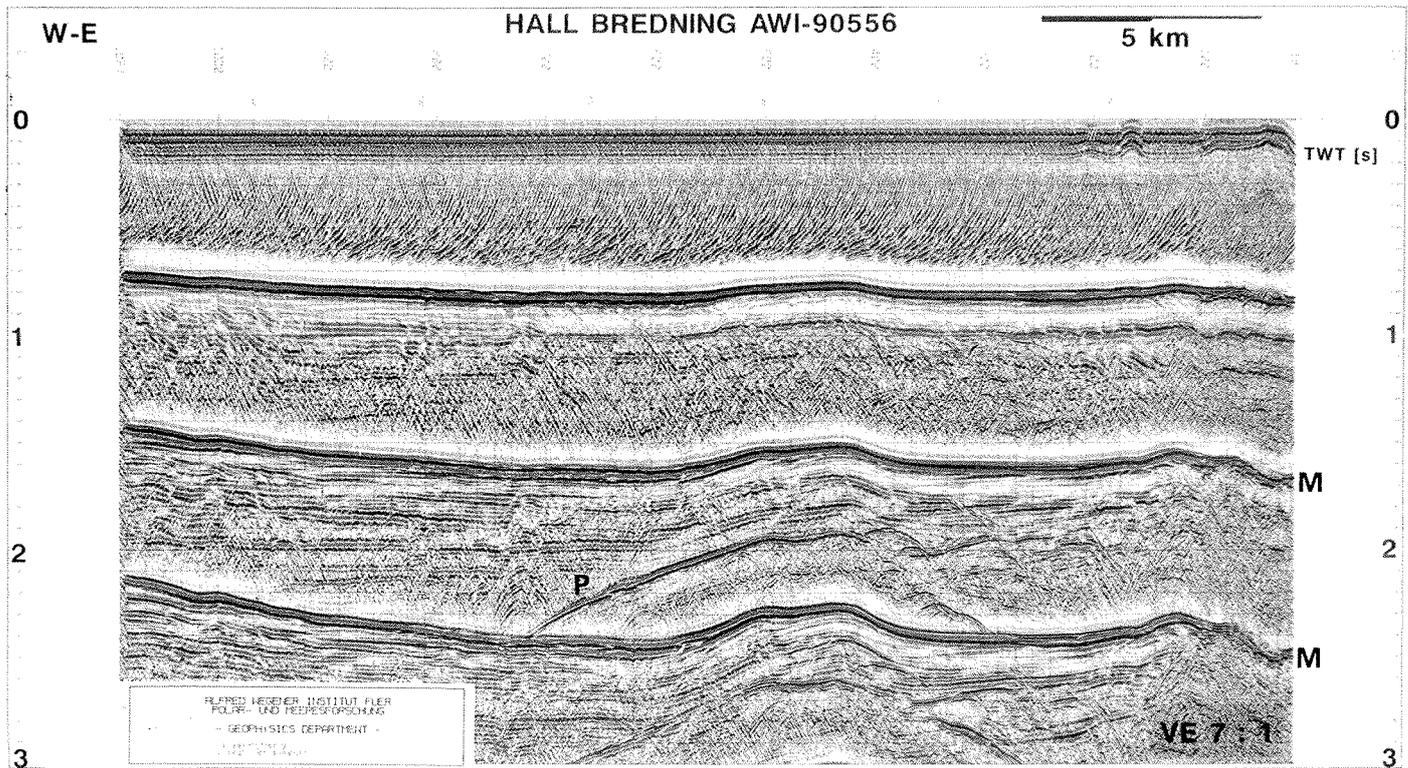
**Fig. 4:** Line AWI-90556 from southwestern Hall Bredning. Here, some deeper structures can be observed in the Mesozoic sequence (between CDP 700 and 100). Those structures may indicate tectonic movements which are restricted to the southwestern part of Hall Bredning and may thus correlate with the western boundary of the Jameson Land Basin. P = primary reflection, M = ocean bottom multiple.
