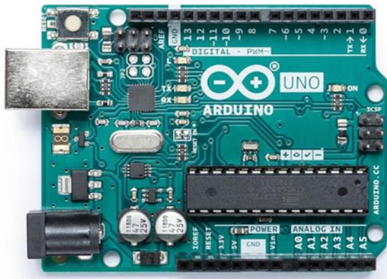
**Fig. 1** Front view of Arduino Uno board. Analog pins are numbered from A0 to A5 (bottom right), whereas digital pins go from 0 to 13 (top row). The symbol “~” denotes pins that can deliver an analog voltage by means of the pulse width modulation (PWM) technique
