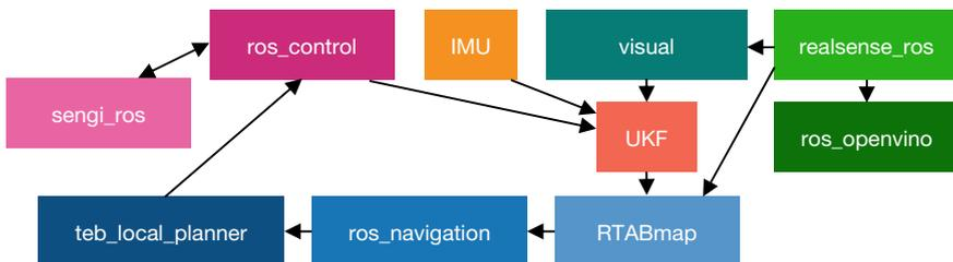
Fig. 3 Simplified diagram of the ROS architecture used in Erwhi Hedgehog
