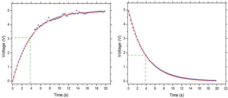
**Fig. 2** Charge (left) and discharge (right) process of an  $RC$  circuit:  $R = 3850 \Omega$  and  $C = 1 \text{ mF}$ . The theoretical time constant is  $\tau = RC = 3.85 \text{ s}$ . The experimental values are, respectively,  $\tau = (3.87 \pm 0.08) \text{ s}$  and  $\tau = (3.83 \pm 0.08) \text{ s}$ . Experimental data (blue dots) are fitted with an exponential curve (red solid line)
