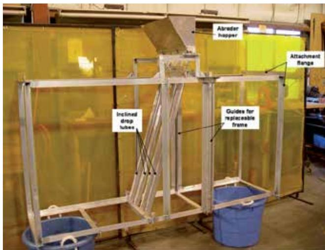
**Figure 3.** A complex flow conditioning section showing the abraded hopper and inclined tubes used to initiate saltation into the flow stream.
