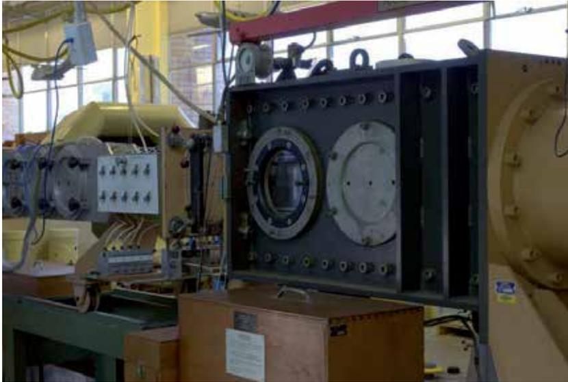
**Figure 2.** A side view of the 5 ½ inch x 4 inch Supersonic Wind Tunnel
