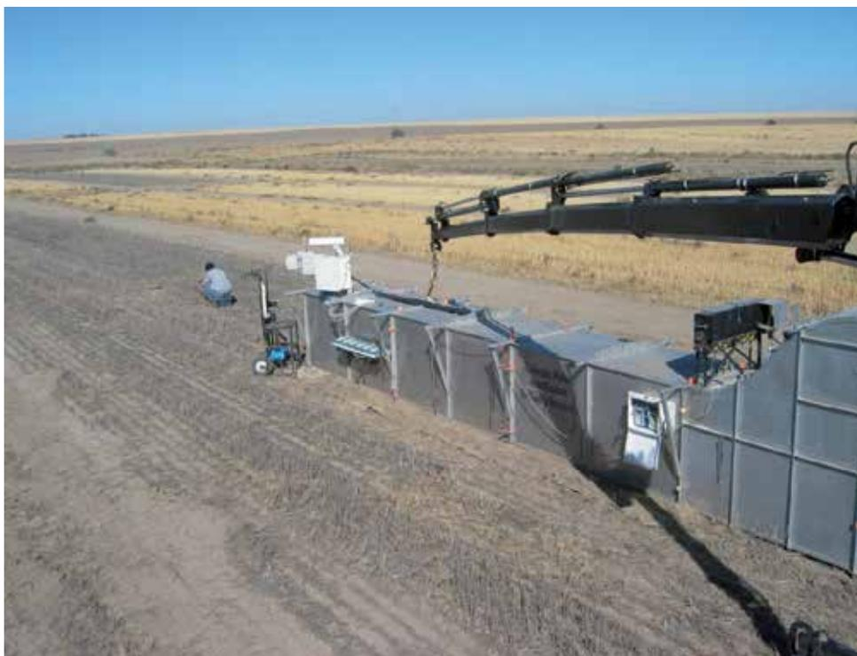
**Figure 2.** A large wind tunnel working section being lowered into place by a hydraulic arm.
