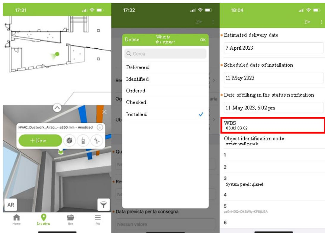
Figure 3. From left to right: (a) Selection of the object the completion of the Status Notification is referred to. (b) Multiple-choice responses to indicate the object's status. (c) Properties of the BIM object, automatically collected from the model: the WBS code is highlighted.
