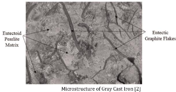
Figure 2. Microstructure of gray cast iron [2].
