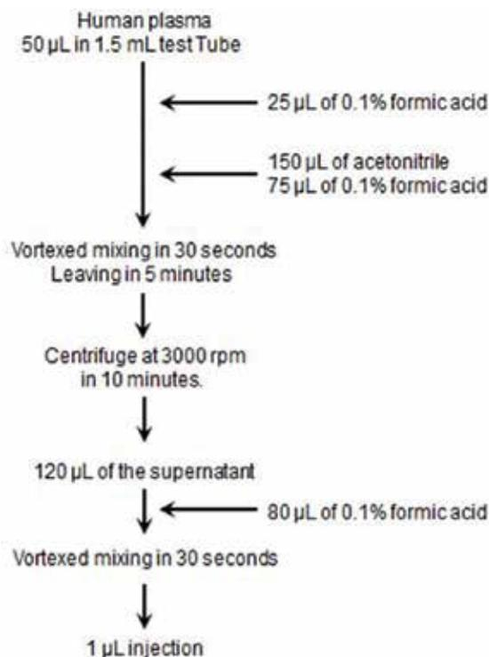
**Figure 1.** The procedure of deproteinization.
