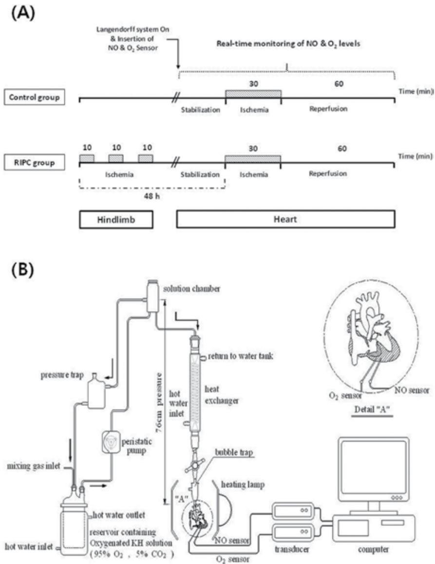
**Figure 3.** Schematic diagrams of (A) experimental design and (B) experimental setup of an isolated heart perfusion system and a real-time monitoring system for nitric oxide and oxygen tension dynamics during myocardial ischemia-reperfusion of the rat. Reproduced from Kang et al. [65]. © 2013 Elsevier B.V.
