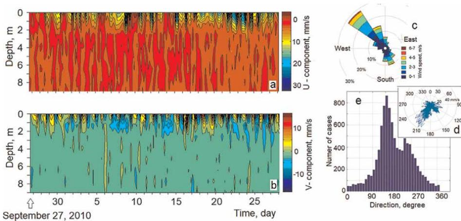
**Figure 7.** Zonal (a) and meridional (b) components of the currents were measured by the acoustic doppler profiler (ADP) in mooring 4, located in El sol Lake. The wind rose from the NMS station data is shown in (c), while (e) displays a histogram of the directions of the currents in the upper 1-m water layer. Additionally, a vector histogram of the same data is presented in (d).
