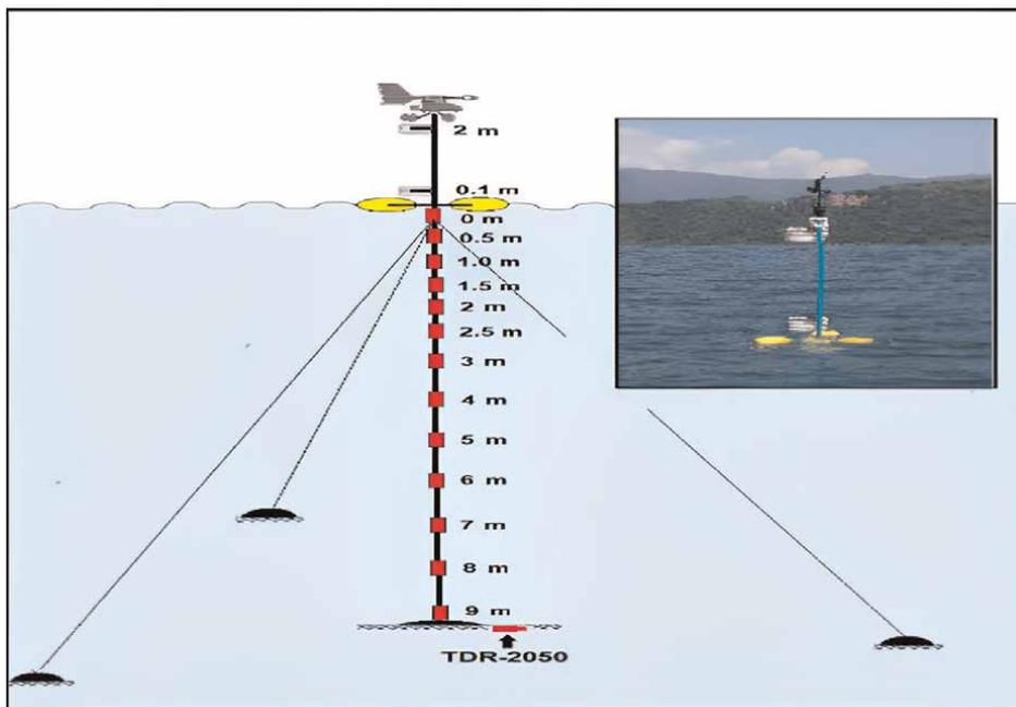
**Figure 3.** Structural scheme of a floating weather station. The photograph in the right corner shows the part of the station above the water level.
