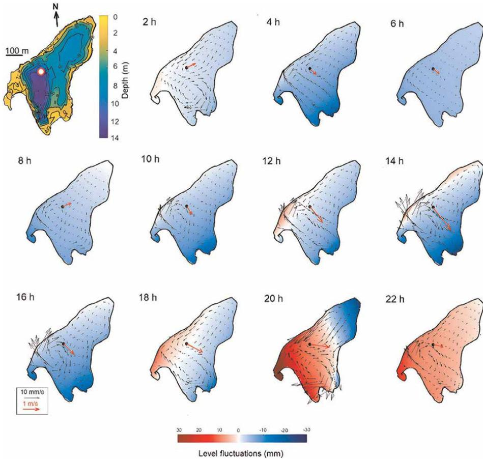
**Figure 9.** Modeling results of current and water level fluctuations in Lake El Sol based on observations taken on September 5, 2018. The rectangles illustrate the simulated currents and level fluctuations for every 2 hours. The black and red patterned arrows in the lower left corner represent the scales for current velocities and measured wind, respectively.
