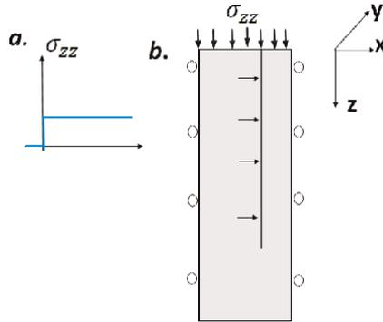
**Figure 4.** This figure, derived from the work of Belferman et al. [44], illustrates the model used in this study. (a) A step-function water load, applied on a top boundary of the structure, representing a poro-elastic seabed; (b) schematic of the structure below the lake with a vertical fault oriented along the outplane axis  $y$ . the calculations are based on uniaxial strain conditions.
