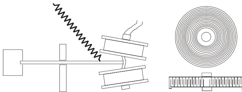
**Figure 5.3:** Schematic sketch on beam damping (right end of beam with hose for air pump) and box for capacitive beam position measurement (left end of beam) plus top and side cut view of an air damper.
