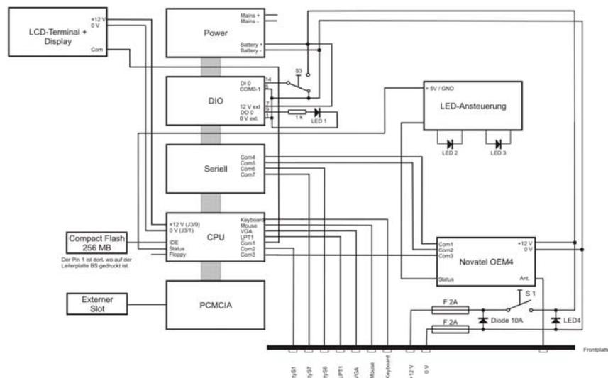
Figure 6.2: Internal architecture of the GFZ GPS ground reference stations.
