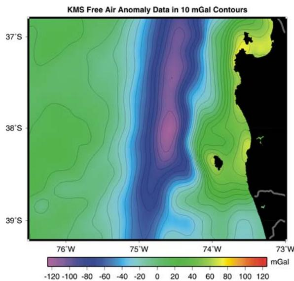
**Figure 10.1:** Free-air anomalies from the KMS'99 model plotted in 20 mGal contour distances.
