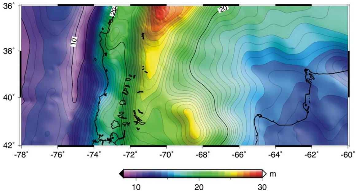
**Figure 14.3:** Gravimetric/altimetry geoid solution for the Southern Andes. Contour lines are drawn at every 1m.
