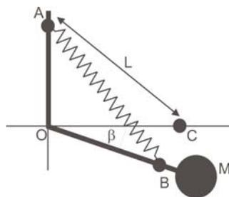
**Figure 5.1:** Simplified principle of a zero-length suspension system: The mass  $M$  is attached to the moveable beam  $OB$  that is free to rotate about  $O$ . The beam is supported by a zero-length spring attached at the points  $A$  and  $B$ . In practice, the beams total travel distance between top stop and bottom stop is about some mm in the Model S meter.
