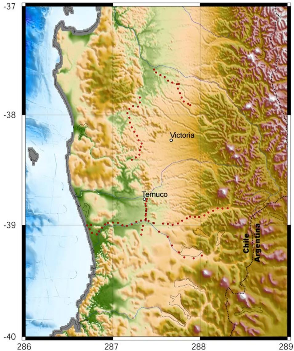
**Figure 13.1:** Location of measured gravity data points (black circles) and absolute gravity stations (white circles) on a shaded-relief map of the working area. Contour lines are drawn in 200 m intervals.
