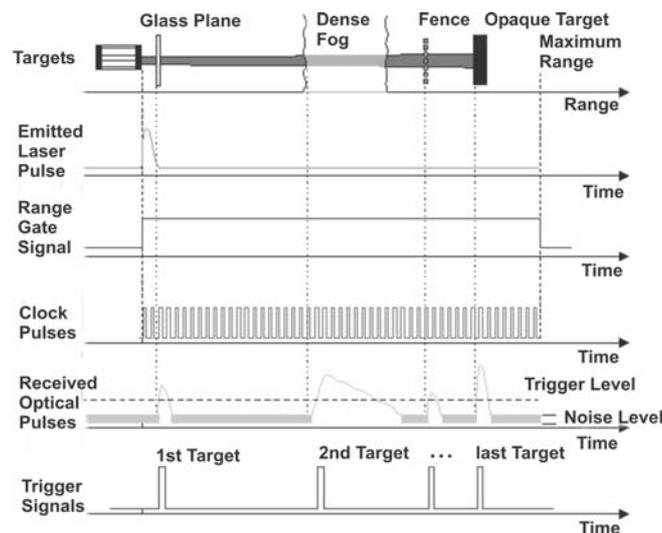
**Figure 5.11:** Last Pulse Detection
