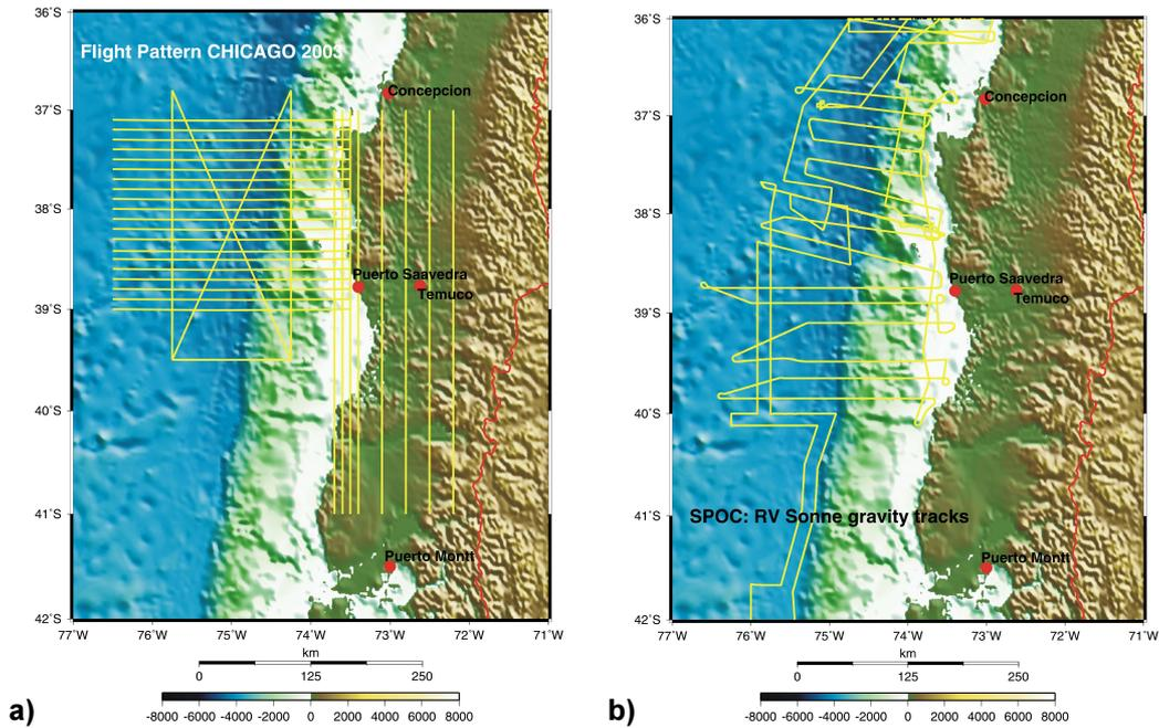
**Figure 1.6:** a) right: Flight lines of the CHICAGO aerogravimetric survey. b) left: Marine track lines from the SPOC survey with RV Sonne.
