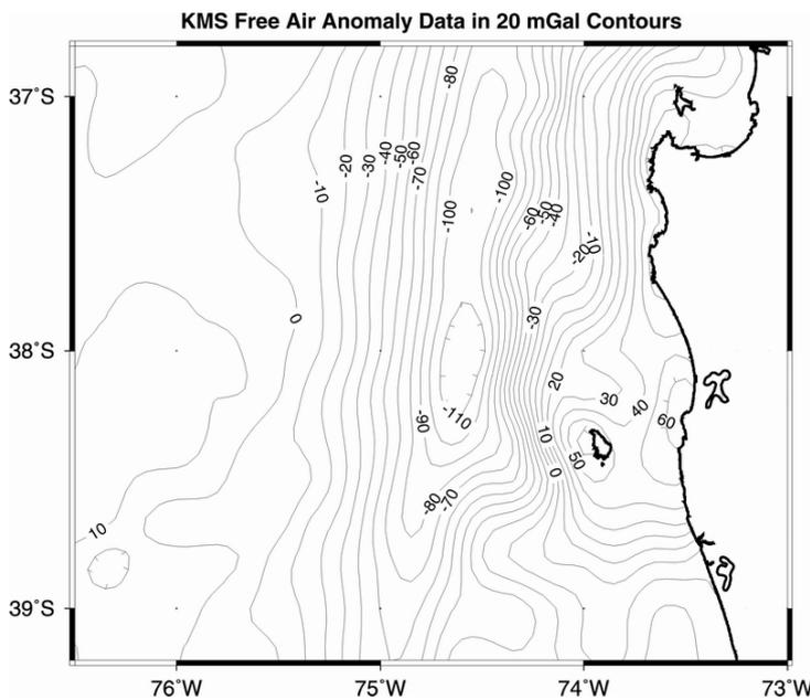
**Figure 8.2:** KMS'99 free-air gravity data contours based on a 3' x 3' grid cell size.
