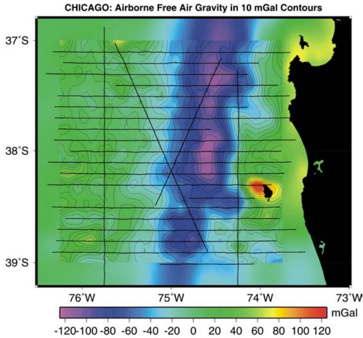
**Figure 10.3:** CHICAGO free-air anomalies plotted in 20 mGal contour distances. Flight lines are given as gray lines in the background.
