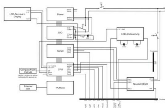
**Figure 5.9:** Novatel OEM4 GPS receiver embedded in the PC104 computer system.
