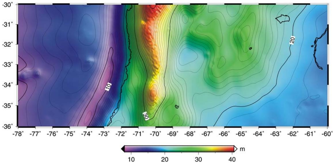
**Figure 14.2:** Gravimetric/altimetry geoid solution for the “metropolitan” area around Santiago. Contour lines are drawn at every 1 m.
