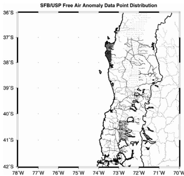
**Figure 9.1:** Distribution of the land based free-air anomaly data points. 11950 points were supplied by the SFB-267 database and 880 points were extracted from the gravity database of the University of Sao Paulo.
