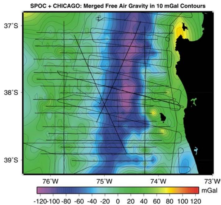
**Figure 10.4:** CHICAGO and SPOC merged free-air anomalies plotted in 20 mGal contour distances. Airborne and marine profiles are given as gray lines in the background.
