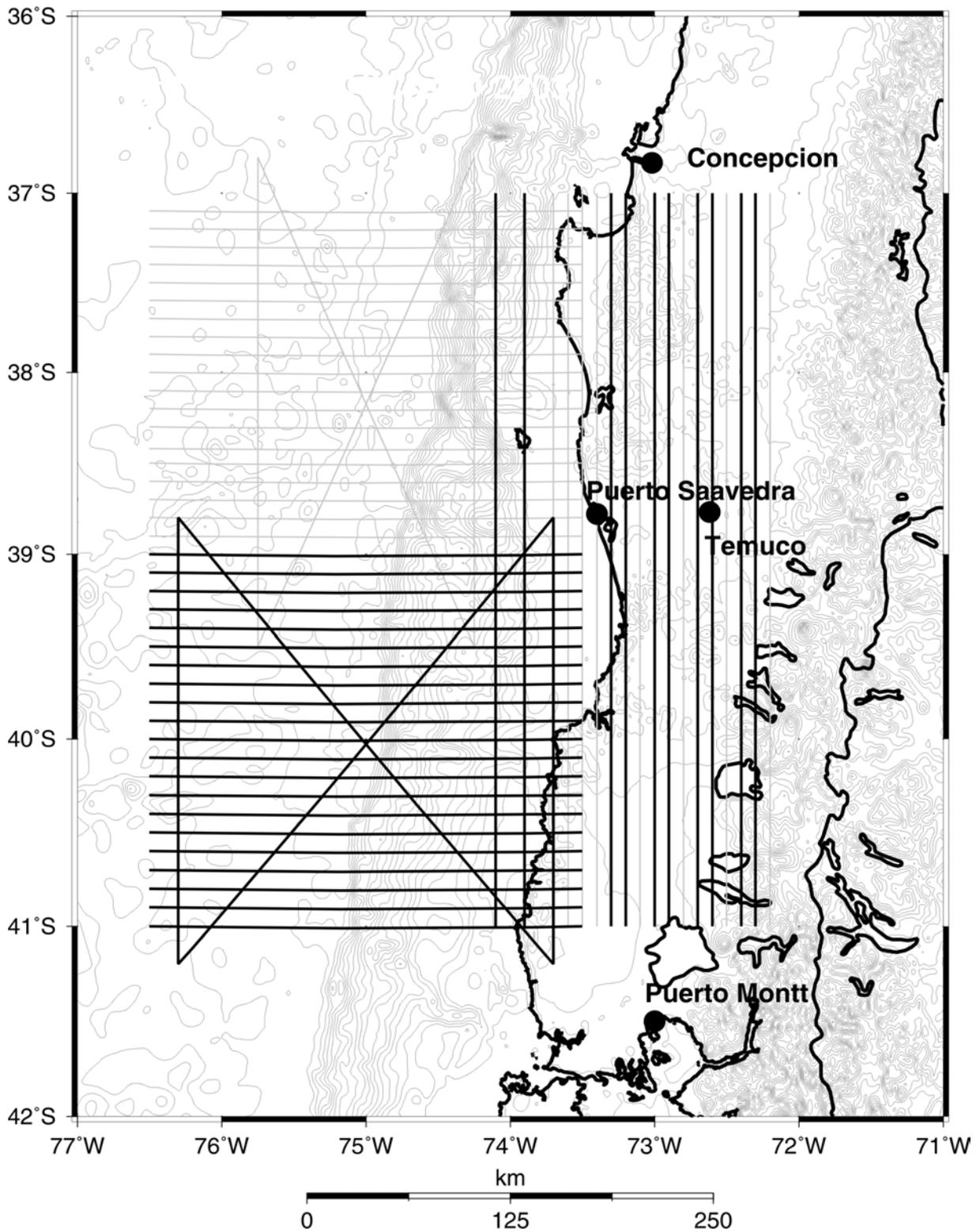
**Figure 11.1:** CHICAGO survey lines as planned to survey in 2004 (black lines). Topographic structures are mapped with 200 m contour lines. The survey profiles from 2002 are given in gray lines.
