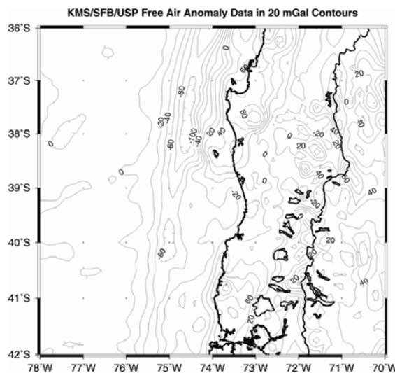
**Figure 9.2:** Free-air anomaly map based on KMS'99 offshore free-air data and the land based data shown in Figure 9.1.
