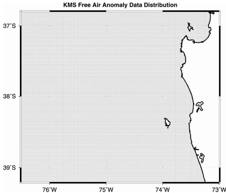
**Figure 8.1:** KMS'99 free-air gravity data distribution. The data was interpolated to a regular 10' x 10' grid cut off by a land-mask defined by the shown shoreline from GMT.
