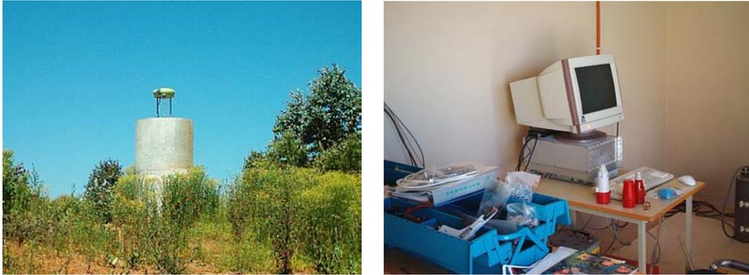
**Figure 6.5:** left: GPS antenna and tower base; right: PC data acquisition unit for 10 Hz GPS data
