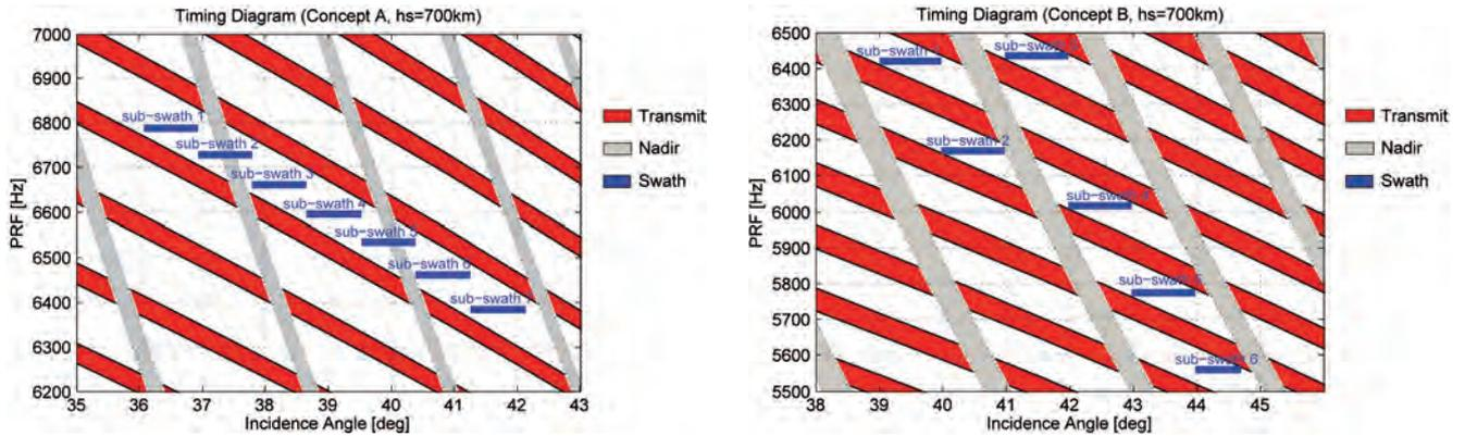
Figure 7.1. Timing examples for 700 km altitude, Concept A is shown on the left and Concept B on the right. Red represents transmission periods, blue reception periods, and grey nadir returns.
