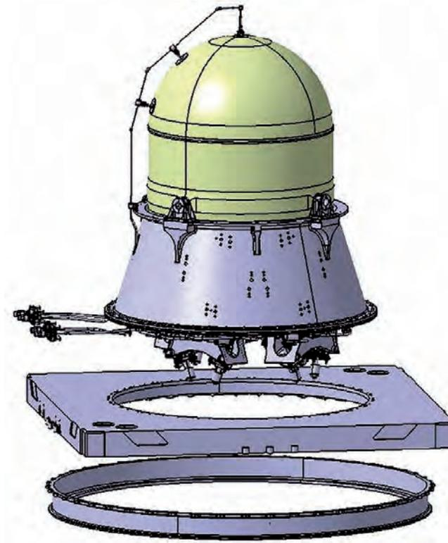
Figure 5.39. CoReH<sub>2</sub>O Concept B thruster assembly.
