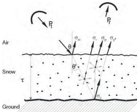
Figure 4.3. Main contributions to radar scattering from snow-covered ground.  $P_t$  is the transmitted power signal and  $P_r$  is the signal that is received by the radar antenna. The angle  $\theta'$  is the angle of refraction in the snowpack. (ENVED)
