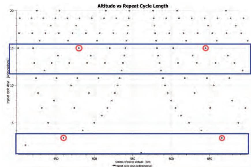
Figure 5.2. Orbit altitude vs. repeat cycle trade-off – only two orbit pairs are suitable.
