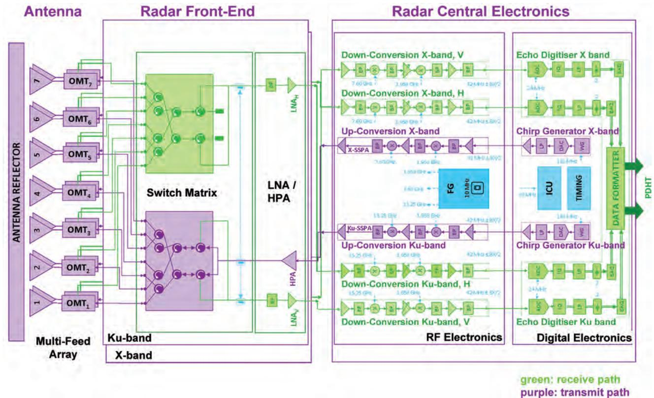
Figure 5.1.1. SAR detailed functional architecture implementation, Concept B.
