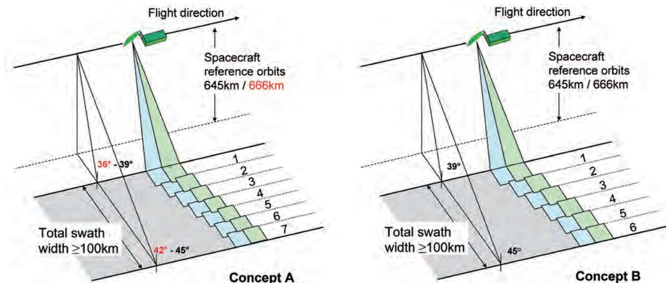
Figure 5.9. Observation principle of the two concepts: ScanSAR acquisition with seven sub-swaths, incidence angles in red for Phase-1 and in black for Phase-2 (left) and ScanSAR acquisition with six sub-swaths, constant incidence angle (right).
