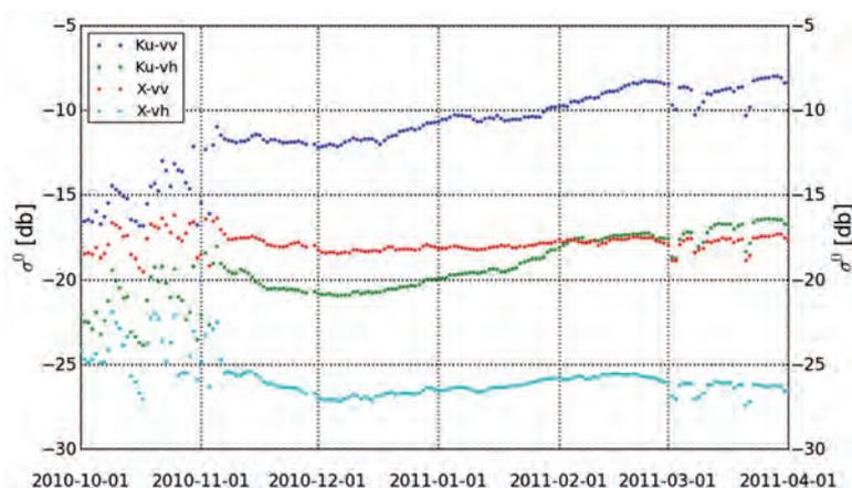
Figure 7.21. Daily averages of X- and Ku-band, VV- and VH-polarised backscatter coefficients  $\sigma^0$  measured by SnowScat at  $40^\circ$  incidence angle during the NoSREx campaign 2010–11. The variation of  $\sigma^0$  during October is related to melt-freeze cycles of soil. Dips in  $\sigma^0$  on several days in March are caused by temporary melt of the snow surface. (ENVEO)
