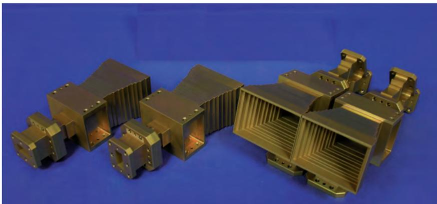
Figure 5.18. Ku-band feed horn element breadboard applicable for CoReH<sub>2</sub>O for Concept B. (Thales Alenia Space IT)
