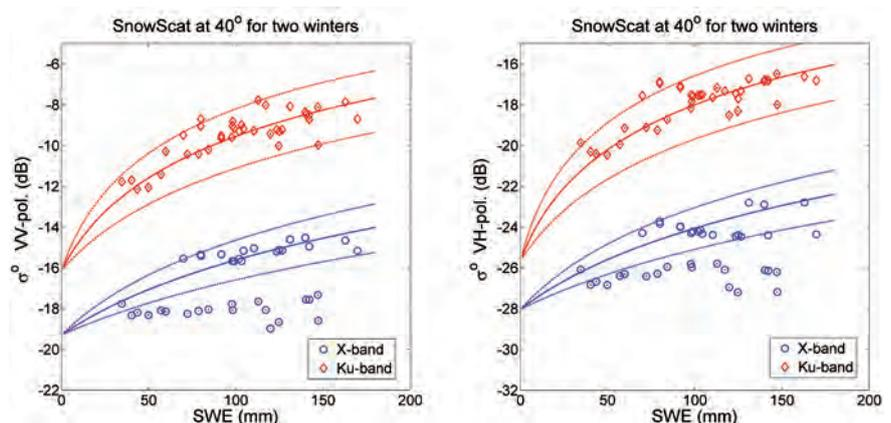
Figure 4.6. Backscatter coefficients as function of observed SWE at Ku-band (16.7 GHz) and X-band (10.2 GHz), 40° incidence angle, from observations at Sodankylä, northern Finland, and forward model calculations (lines) for boreal snow conditions. The points correspond to tower-based SnowScat measurements for the winters of 2009–10 (open symbols) and 2010–11 (dotted symbols). (FMI)
