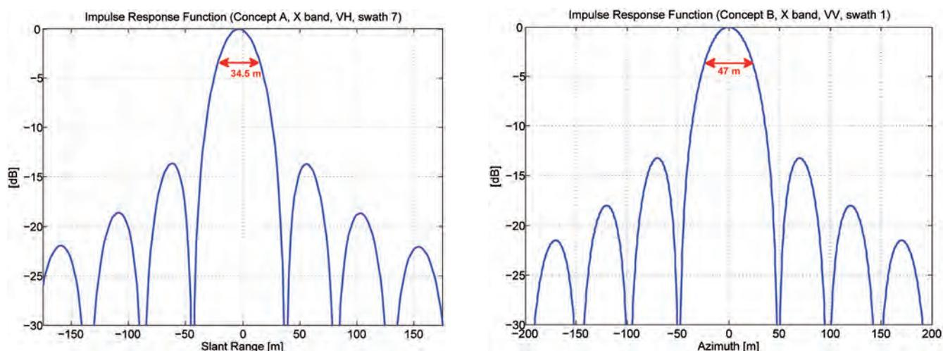
Figure 7.4. X-band IRF examples with windowing in slant range (left: Concept A, swath 7) and azimuth (right: Concept B, swath 1).
