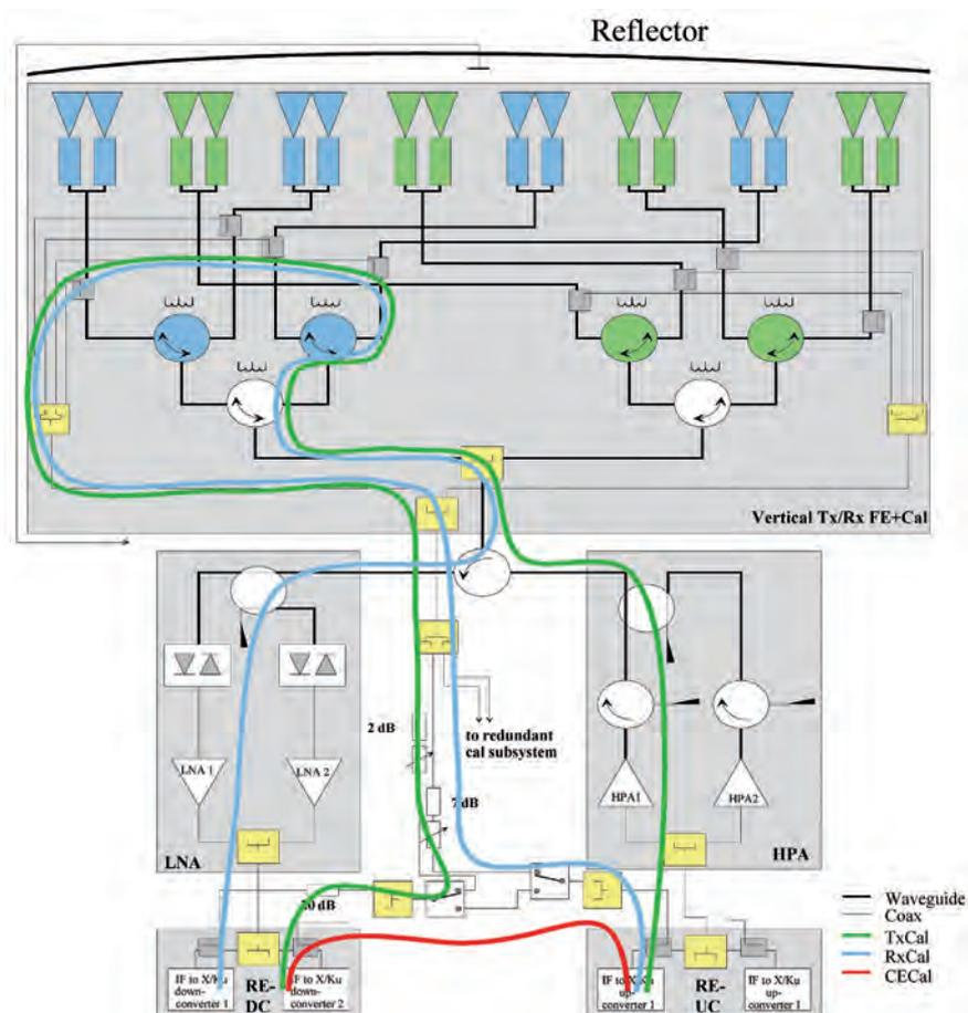
Figure 5.25. Front-end block diagram showing calibration loops for V path as defined for Concept A.
