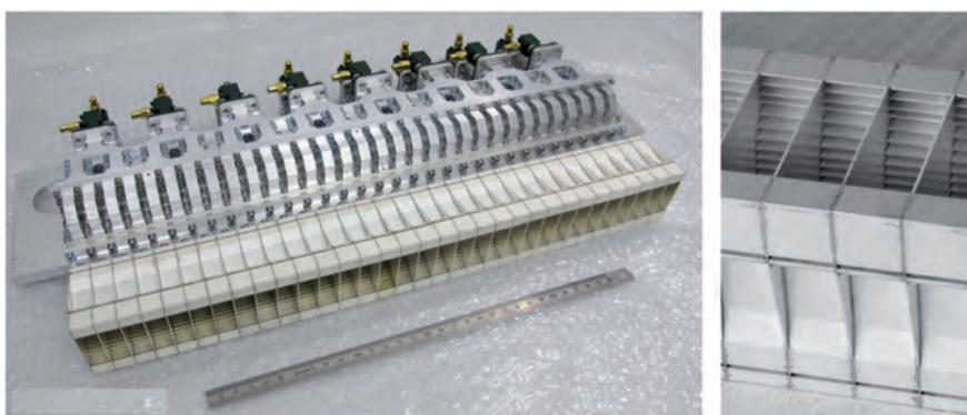
Figure 5.15. Concept A Ku-band MFA breadboard applicable for CoReH<sub>2</sub>O. (EADS Astrium GmbH)
