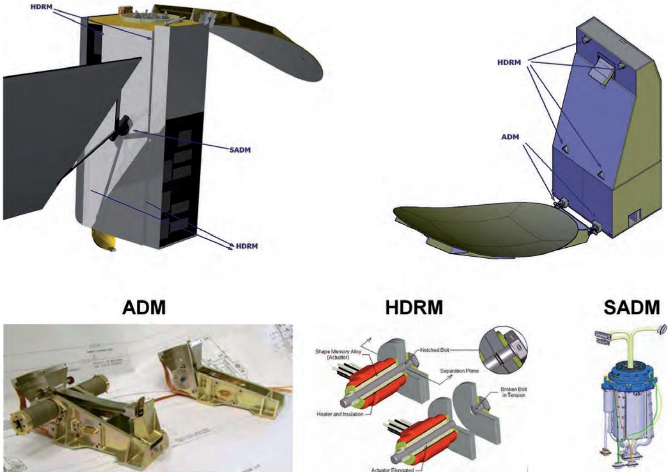
Figure 5.32. CoReH<sub>2</sub>O mechanism locations (top) and implementation (spring for ADM bottom left, Frangibolt for HDRM bottom middle, and for rotary joint as a part of the SADM, bottom right). (Lower centre image: TINI Aerospace)
