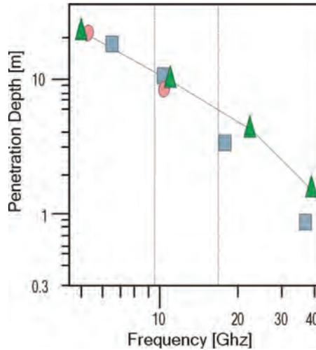
the penetration depth in the X- to Ku-band range is in the order of several metres, increasing from values of 3–4 m at 17.2 GHz to about 10 m at 9.6 GHz (Fig. 4.2).
