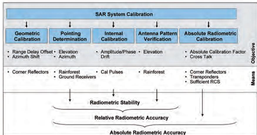
Figure 5.26. SAR system calibration procedures required for the absolute radiometric calibration of the SAR data products.
