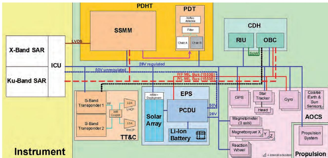
Figure 5.33. Electrical architecture (example for Concept A) showing the interfaces.
