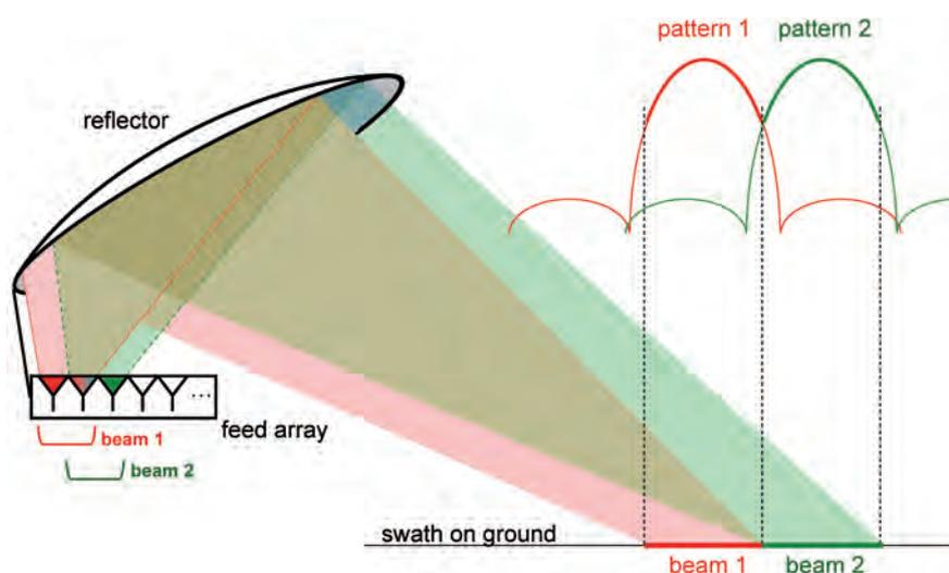
Figure 5.14. The antenna multiple-beam feed horns approach to form the ScanSAR beams.
