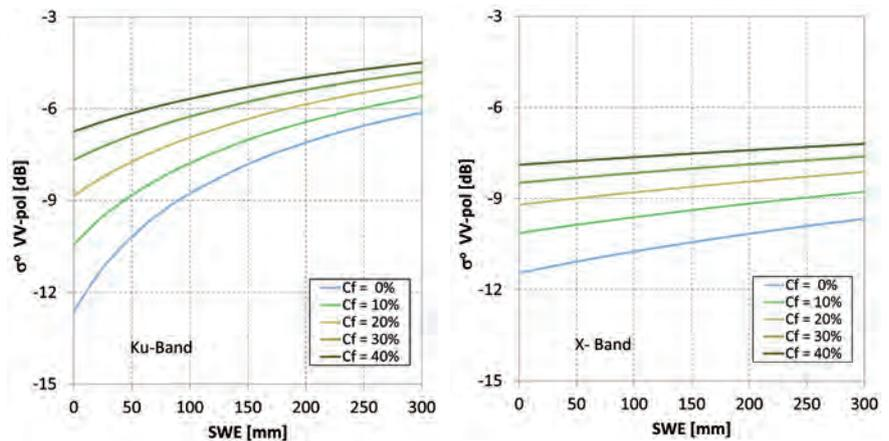
Figure 4.8. Simulated backscattering coefficients for forest canopy (coniferous forest) and snow-covered ground as a function of SWE at 17.2 GHz (left) and 9.6 GHz (right), VV polarisation, incidence angle 40°, for forest Cover Fraction (CF) from 0% (non-vegetated surface) to 40%. Woody volume of the forested area ranges 0–350 m<sup>3</sup>/ha. (IFAC)
