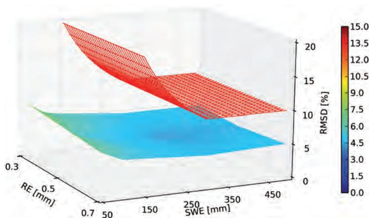
Figure 7.16. Relative root mean square difference (RMSD relative to the mean) between retrieved and true value of SWE for open land, basic test.  $R_e$ : effective grain radius of snow; SWE: snow water equivalent. The red grid indicates the benchmark for the SWE product ( $\pm 30$  mm for SWE  $\leq 300$  mm,  $\pm 10\%$  for SWE  $> 300$  mm). (ENVEO)
