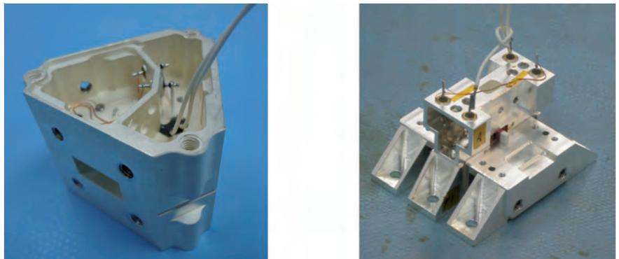
CoReH<sub>2</sub>O is smaller, but the power has to be increased. A model of the phase shifter has already been built and successfully tested (Fig. 5.21 right).
