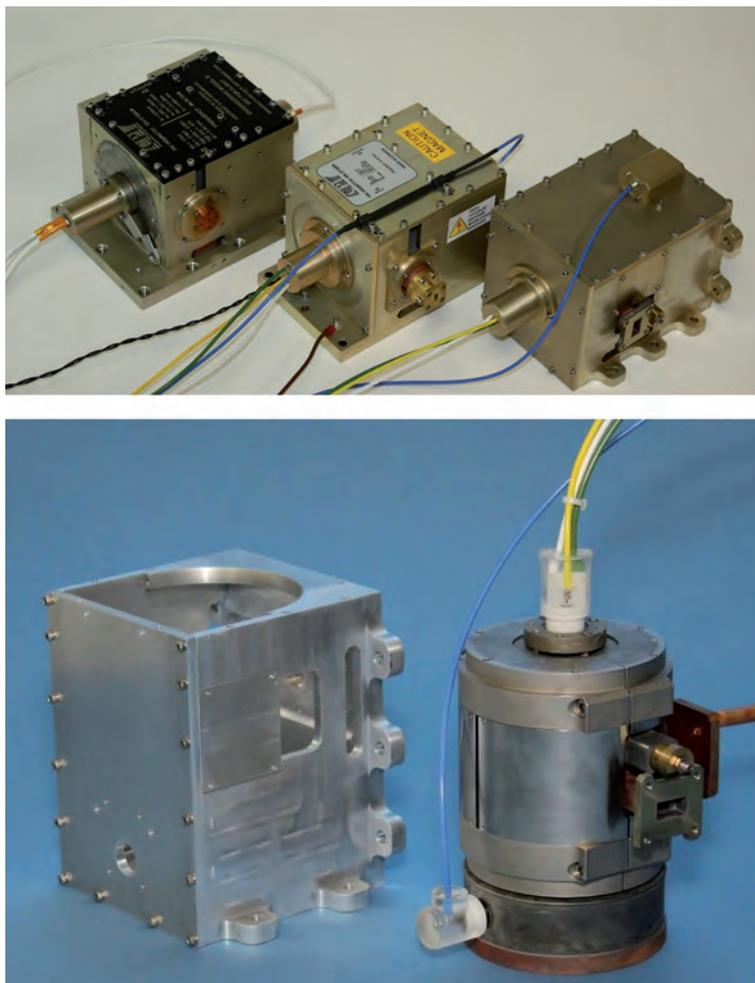
Figure 5.24. Klystron models. Top left to right in decreasing order of operating frequency: EarthCARE model (94 GHz), SWOT model (35 GHz), first Ku-band EM for CoReH<sub>2</sub>O (17.2 GHz). Bottom: Ku-band EM before enclosure. (CPI Inc.)
