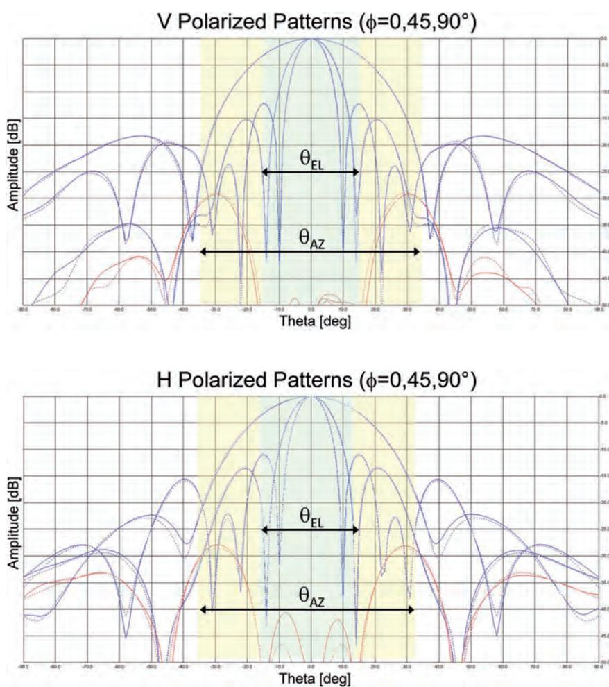
Figure 5.19. Comparison between measured and simulated primary patterns at feed level (simulated dotted line, measured continuous line) for Concept B feed breadboard.
