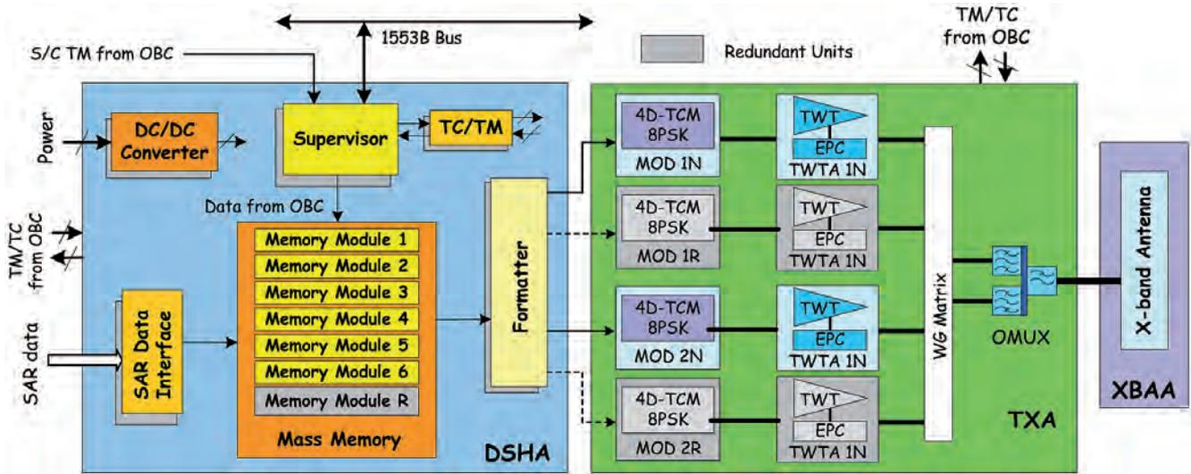
Figure 5.34. PDHT subsystem design (Concept B).
