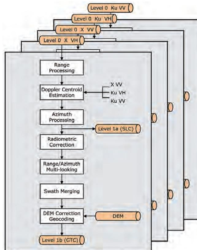
Figure 5.43. Processing chain for CoReH<sub>2</sub>O Level-1b products.
