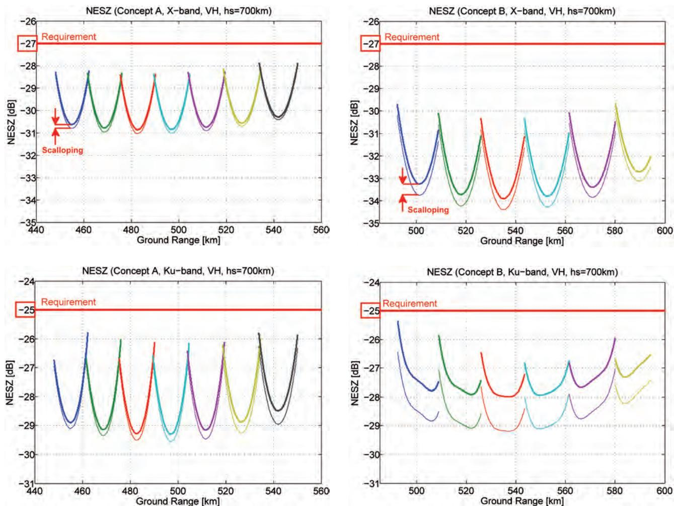
Figure 7.6. NESZ curves (VH, 700 km) for X-band (top) and Ku-band (bottom) for Concepts A (left) and B (right), showing all six or seven sub-swaths.
