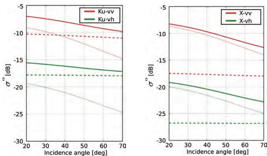
Figure 4.5. Model calculations of the total backscatter (solid line) dependent on incidence angle, and contributions of the snow volume (dashed) and rough soil surface (dotted). For seasonal snow with SWE=150 mm at 17.2 GHz (Ku-band) and 9.6 GHz (X-band); co-polarisation (VV), cross-polarisation (VH). (ENVEO)
