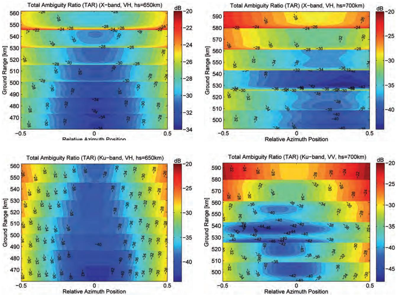
Figure 7.7. TAR curves for X-band (top) and Ku-band (bottom) for Concepts A (left) and B (right).
