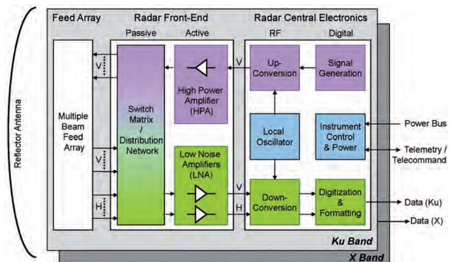
Figure 5.10. Payload functional architecture.
