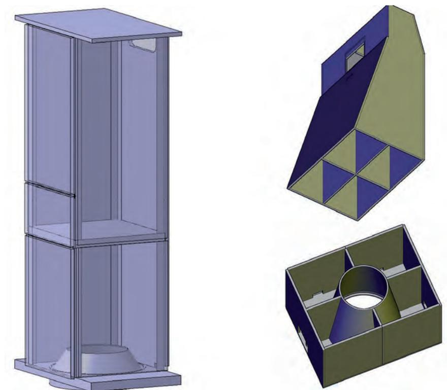
Figure 5.28. Panel-based structural concept (Concept A left, Concept B right).
