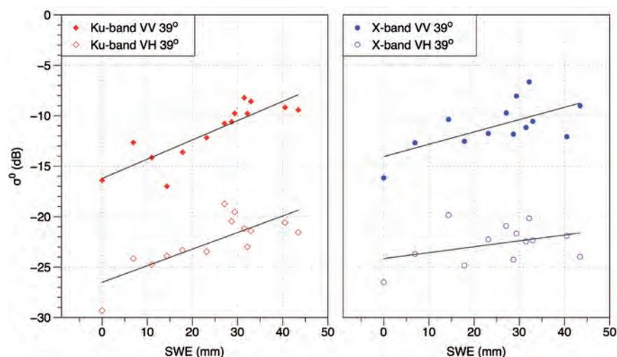
Figure 4.7. Behaviour of backscatter (normalised radar cross-section) as a function of SWE for the wet tundra site of Churchill, at X- and Ku-bands. The results show a strong correlation between the radar observations and SWE. (University of Waterloo)
