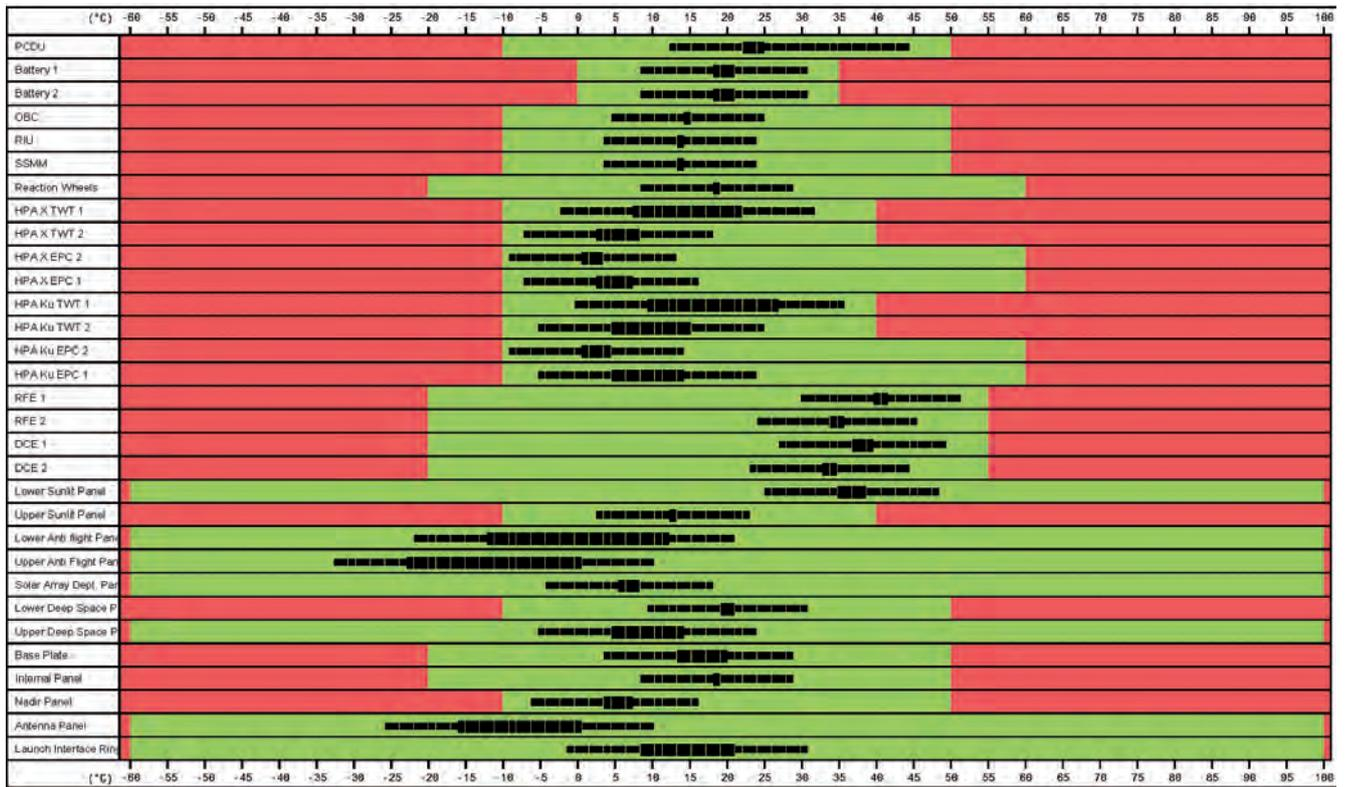
Figure 5.31. Temperature predictions for equipment for Concept A (predicted/operating range in black/green).
