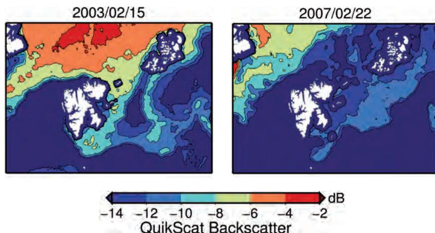
Figure 4.11. Ku-band (QuikSCAT) backscatter maps of the Barents Sea for two dates in February 2003 and 2007, showing large differences related to sea-ice type. High backscatter (red) coincides with rough multiyear ice, low backscatter (blue) with smooth first-year sea ice. (Adapted from Hendricks et al., 2011)
