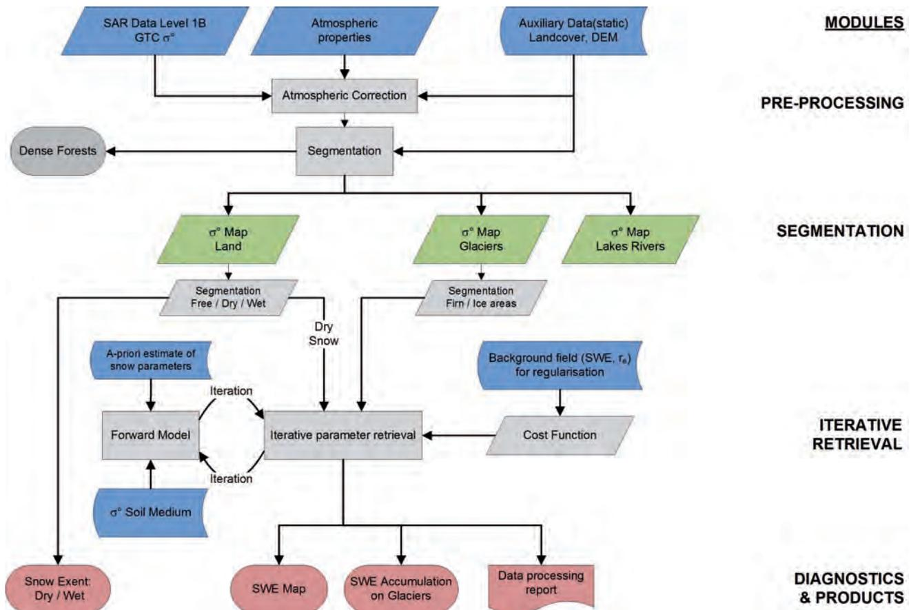
Figure 6.1. CoReH<sub>2</sub>O processing line for retrieval of basic Level-2 products. (ENVEO)
