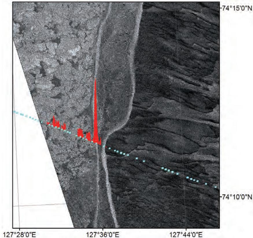
Figure 2.15. Coastal polynya, Laptev Sea. Subset of the TerraSAR-X stripmap scene, X-band, HH, 28 April 2008, with thickness profile overlay. The dark grey area in the right of the image is the new ice with a fraction of open water. Light grey bands represent the border where the young ice hits the consolidated pack ice. The left part of the image is the consolidated ice zone, with bigger floes. (Adapted from Busche et al., 2009)
