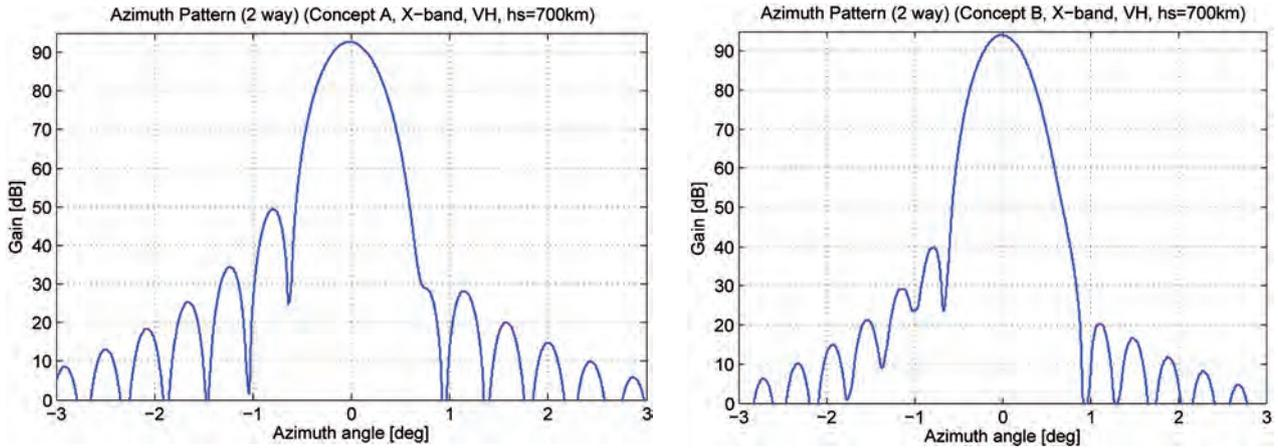
Figure 7.3. Example azimuth antenna pattern for beam-1. Concept A is shown on the left and Concept B on the right.
