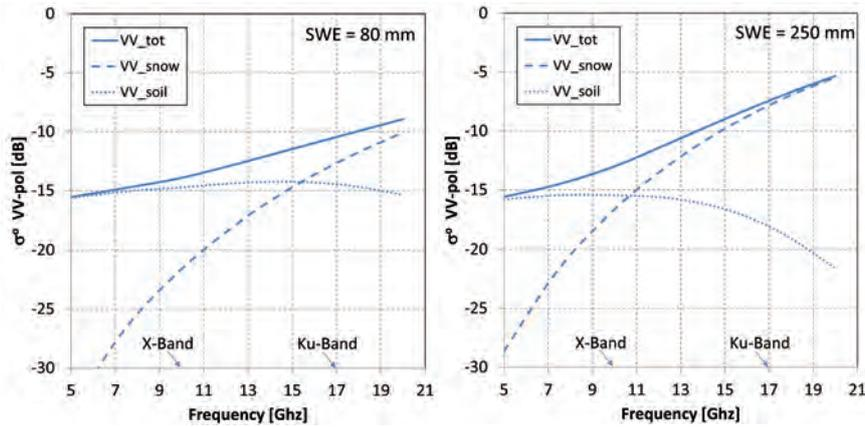
Figure 4.4. Backscatter coefficients at VV polarisation ( $40^\circ$  incidence angle) for shallow (SWE=80 mm, left) and deep snow (SWE=250 mm, right) over a moderately rough soil background. Solid line=total backscattering, dashed line=snow volume contribution, dotted line=soil contribution attenuated by snow. (IFAC)
