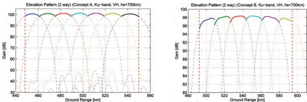
Figure 7.2. Overlapping elevation antenna patterns of different sub-swaths projected on the ground. An example of Ku-band for Concept A is on the left and Concept B on the right. Beam number increases with increasing range.
