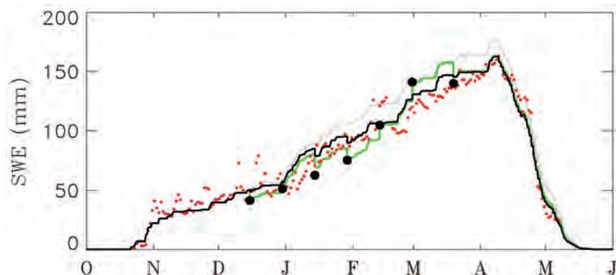
Figure 6.3. Observations and simulations of SWE at Sodankylä in 2010–2011. Red dots show *in situ* measurements and black dots show SWE retrievals based on SnowScat backscatter measurements, thinned to a 15-day repeat cycle. Simulations were run as an open-loop forecast (grey line), with direct insertion of the retrievals (green line) and with assimilation of the retrievals (black line). (University of Edinburgh)
