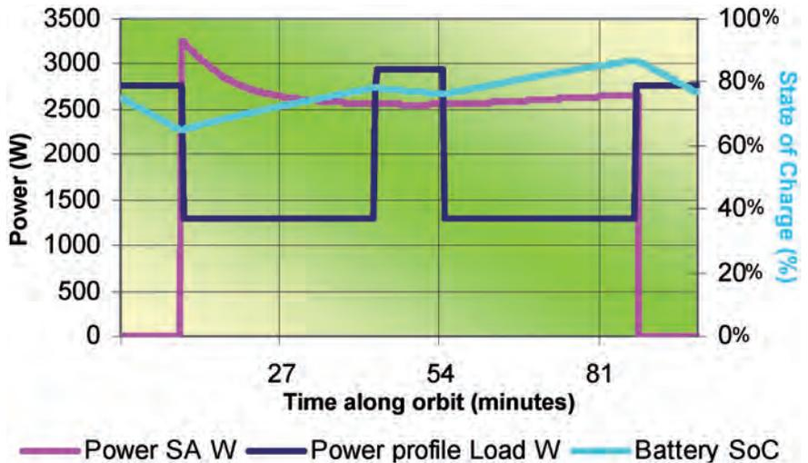
Figure 5.36. Typical power supply & demand profile for one orbit (Concept A).
