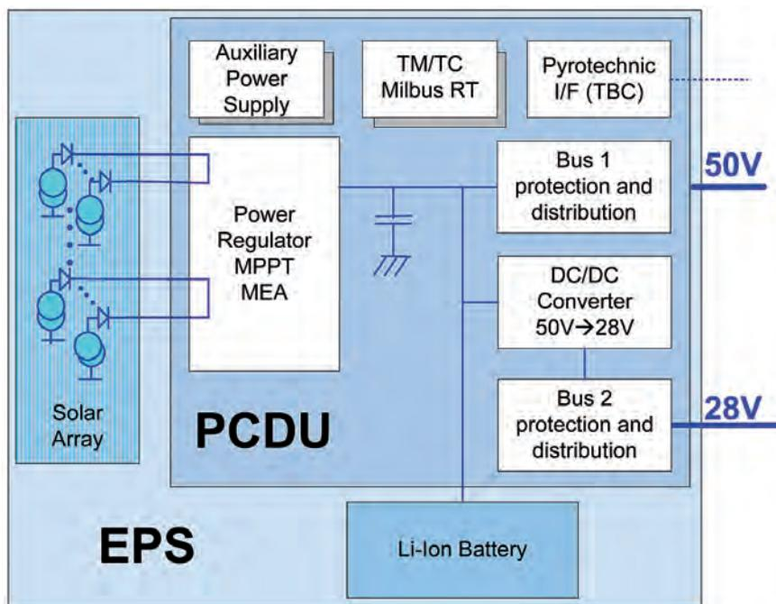
Figure 5.35. EPS block diagram (Concept A).
