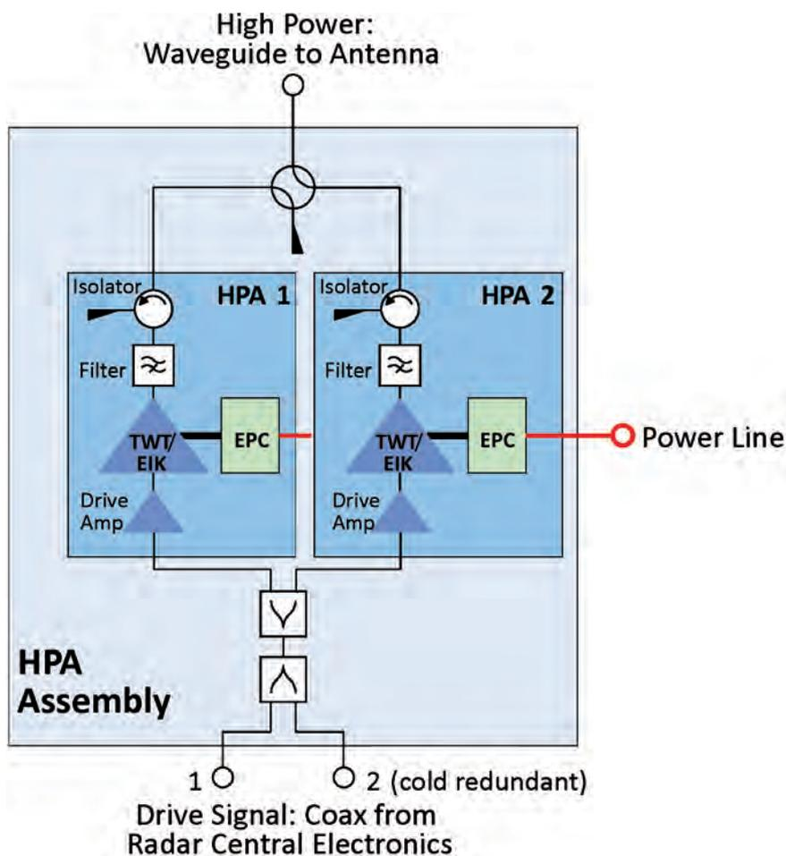
Figure 5.22. Functional block diagram of HPA assembly (per frequency band).
