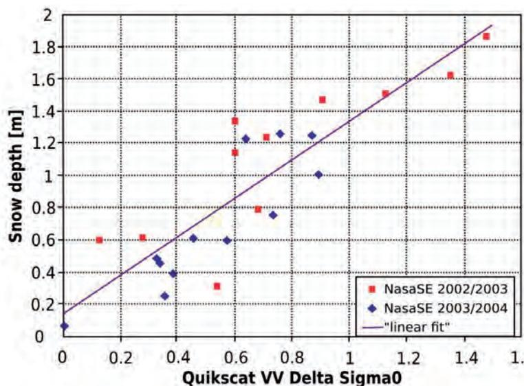
Figure 4.9. Ku-band backscatter difference ( $\Delta\sigma^0 = \sigma^0_{\text{autumn}} - \sigma^0_{\text{winter}}$ ) in dB derived from QuikSCAT data vs. snow depth at the station NASA-SE at 20-day intervals, during accumulation periods 2002–03 and 2003–04. (ENVEO).
