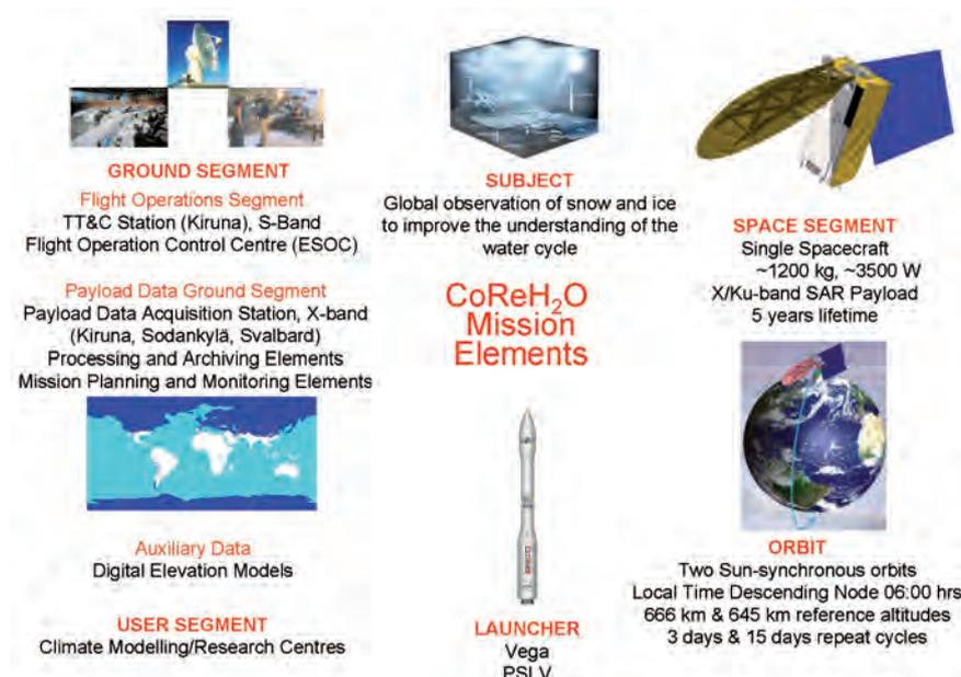
Figure 5.1. CoReH<sub>2</sub>O mission and system architecture.
