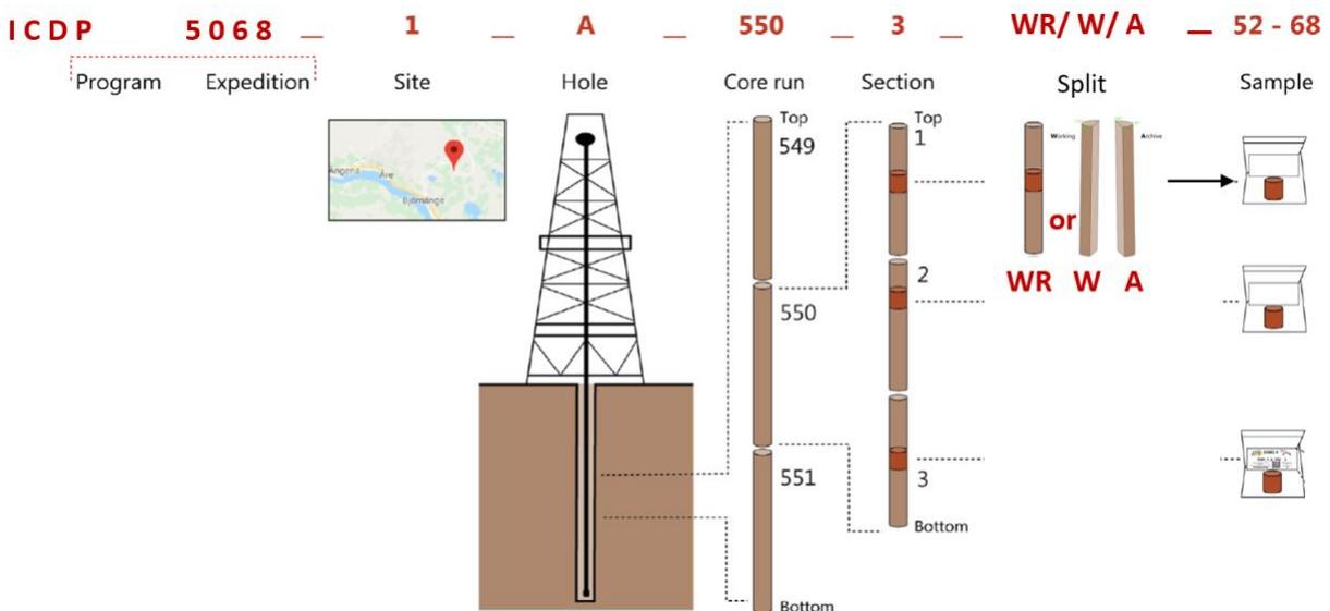
Figure 1 : Example for the common naming convention used in ICDP. The combined\_id is used in ICDP to name any site, hole and drilled or cored material.
