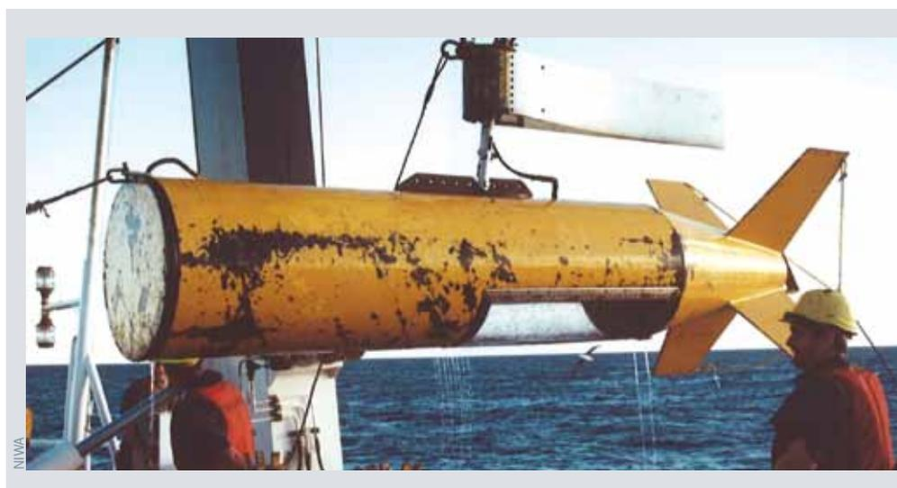
Deploying a deep acoustic towbody from the research vessel *Tangaroa* to survey deep-sea fish stocks off New Zealand. Acoustic surveys are regularly carried out to monitor the size of spawning aggregations of species such as orange roughy and oreo dories.
