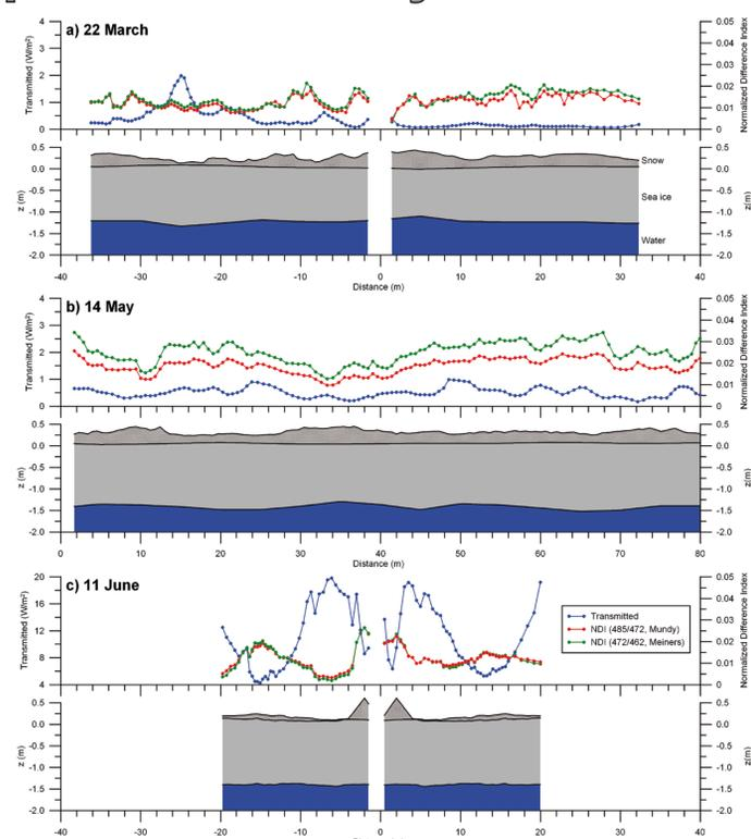
**Figure 4:** Under-ice (transmitted) irradiance and normalized difference index (NDI) along profiles on first-year fast ice off Barrow, Alaska, on (a) 22 March, (b) 14 May, and (c) 11 June 2010. In March and June, two transects were performed away from the same access hole ( $x=0$ ) and are considered as one profile each. The NDIs are calculated as suggested by Mundy et al. (2007) and K. Meiners (pers. comm.). Note the different scaling of transmitted irradiance in (c).
