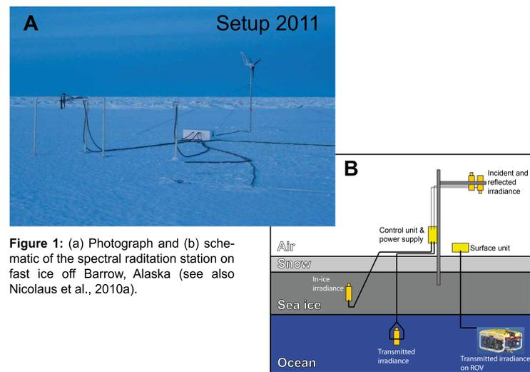
**Figure 1:** (a) Photograph and (b) schematic of the spectral radiation station on fast ice off Barrow, Alaska (see also Nicolaus et al., 2010a).
