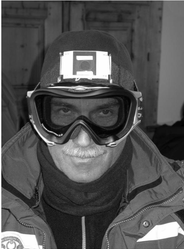
**Fig. 1.** Instructor, dosimeter attached to the cap.
