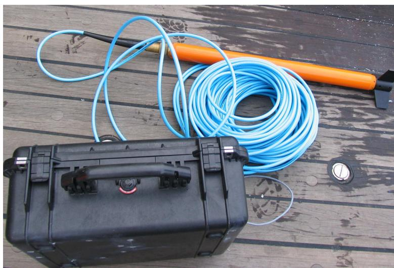
Figure 2.4: Magnetometer
